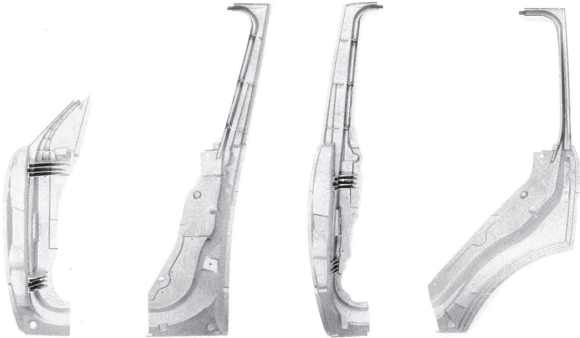
6.17 Inner door panels of a SUV. Weight: 2.0–2.2 kg. Dimensions: ca. 1000 × 240 mm to 1400 × 500 mm. Wall thickness: 2–2.5 mm. Temper: F.
