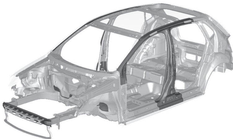
9.12 Hot-formed parts in the body of VW Polo V (Eichhorn, 2009).
