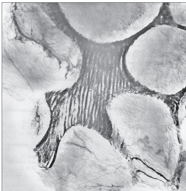
7.5 Analytical electron micrograph of AXJ530 alloy showing primary Mg grains and a grain boundary eutectic structure comprising (\text{Mg},\text{Al})_2\text{Ca} and Mg (Powell et al. , 2001) (used with permission of SAE International).
