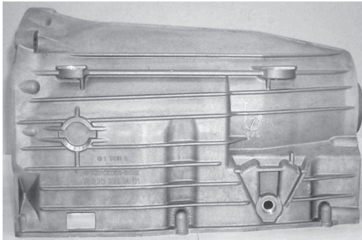
7.17 The Mercedes 7-speed automatic transmission case (after Greiner et al. , 2004) (used with permission of Daimler).
