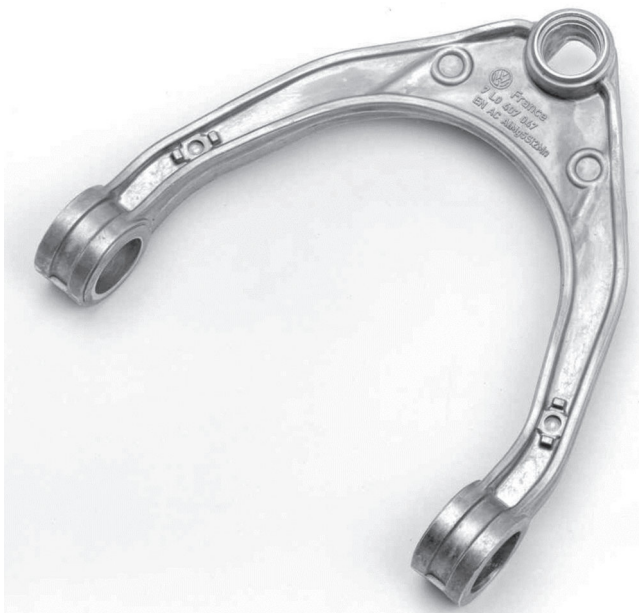
6.23 Suspension strut bracket for SUVs. Weight: 0.9 kg. Dimensions: 340 \times 370 \times 60 \text{ mm} . Wall thickness: max. 6 mm. Temper F.
