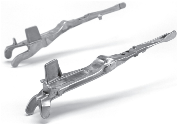
6.32 RHT folding levers of the VW EOS. Weight: 0.56 kg. Dimensions: 510 × 100 × 80 mm. Temper F.
