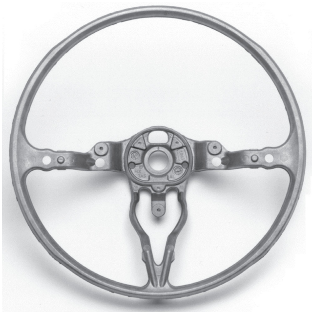
6.22 Steering wheel of the VW Beetle. Weight: 0.85 kg. Dimensions: \text{Ø } 350 \times 125 \text{ mm} . Temper F.
