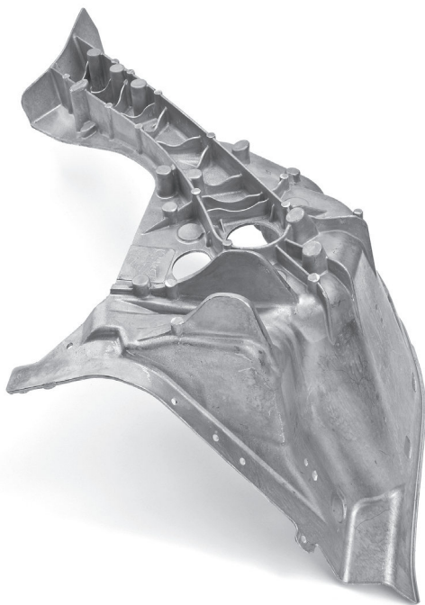
6.19 Shock tower. Weight: 2.3 kg. Dimensions: ca. 500 × 280 × 500 mm. Temper: F.
