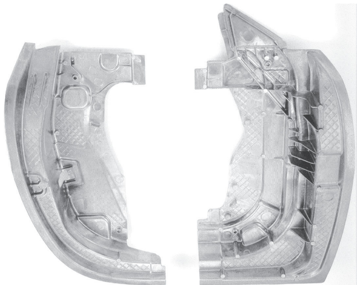
6.29 Hinge and latch door panels of the Jaguar XK. Weight: 1.2 to 2.1 kg. Dimensions: ca. 700 \times 340 \times 170 mm. Temper: O.
