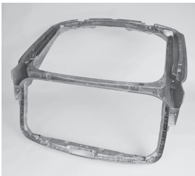
6.7 Rear lid frames of the BMW Series 5 GT. Weight: 11.6 kg. Dimensions: ca. 1230 × 1250 × 390 mm. Temper: F.
