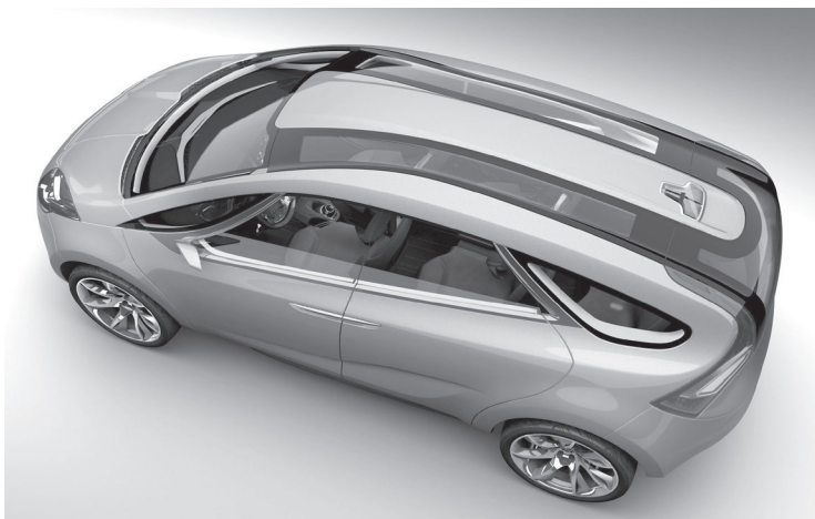
8.9 Polycarbonate glazing of the 'i-mode' concept car. A development between Hyundai and Bayer MaterialScience AG (Bayer AG).
