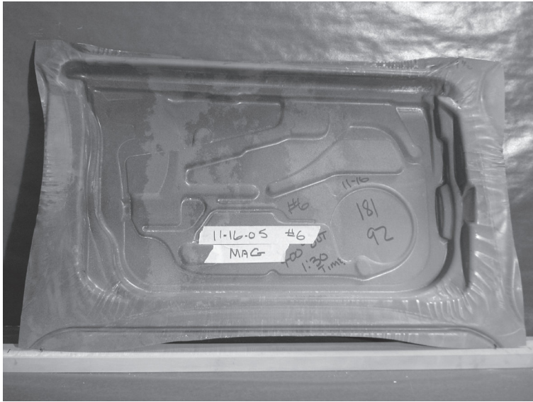
7.25 Magnesium door inner panel made by warm forming (Krajewski et al. , 2006).
