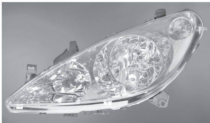
8.8 PBT headlight bezel from the Peugeot 307 (Bluhm et al. , 2008).
