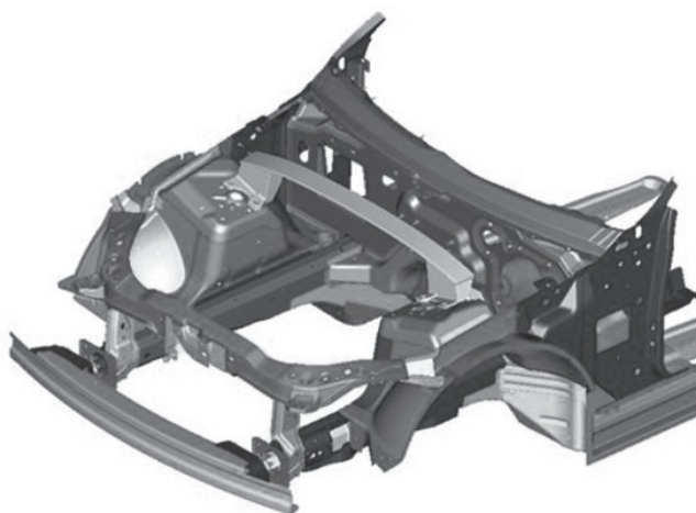
7.20 Schematic of the front end of a production sedan (used with permission from General Motors Inc.).
