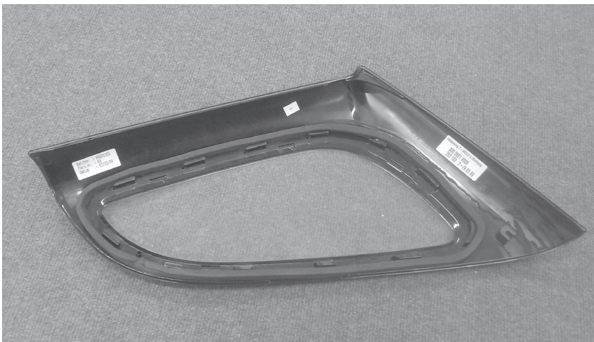
11.3 Integrated components on a Smart ForTwo rear quarter window.
