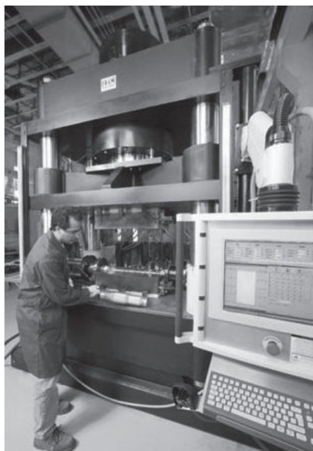
7.37 Warm gas forming press at CANMET, Ottawa, Canada (Martin et al. , 2005).
