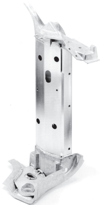
6.5 High-pressure die-casting nodes of the A-pillar in the first ASF of Audi A8. Weight: 4.1 kg. Dimensions: ca. 850 \times 550 \times 90 mm. Temper: T7.
