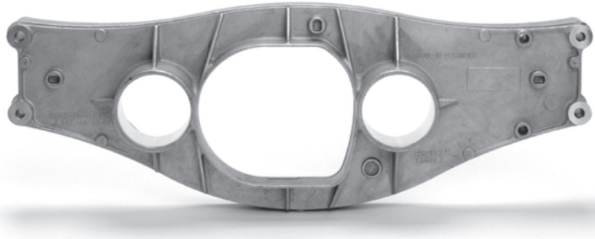
6.21 Gearbox crossbeams of the Mercedes S-Class. Weight: 2.3 kg. Dimensions: 610 × 210 × 75 mm. Temper T5.
