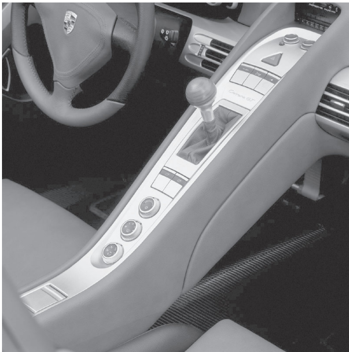
7.26 Sheet magnesium center console cover in Porsche Carrera GT automobile (copyrighted by Dr Ing. H.c. F. Porsche AG. Used with permission).
