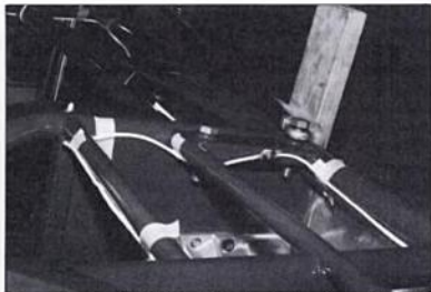
Use masking tape to hold the clothesline in place. If possible, try to represent actual clamps or nylon ties that will hold finished harness in place.
