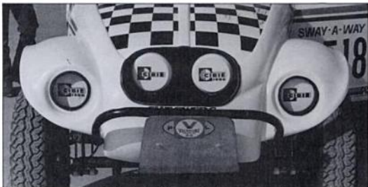
Off-road racers rely on high-output driving and fog lamps to illuminate as much as the terrain as possible. Setup shown here is basic—two headlamps and two driving lamps. Many off-road setups use more lamps than this—mounted in locations to minimize damage during racing—which likely would be illegal for street use. Lens covers protect lamps when not in use—they're also good advertising for lamp manufacturer! Photo by Ron Sessions.
