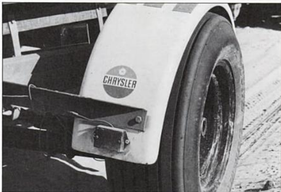
Ground for fender-mounted taillamp relies on metal fender attached to trailer frame, which in turn is attached to tow vehicle through hitch—a shaky ground at best. Better to run separate ground wire from lamp directly to good known ground on tow vehicle. Also note how wires are “hanging” unprotected beneath trailer. Bad wiring job is typical of that found on most trailers. Photo courtesy Trailer Boats Magazine.
