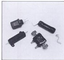
Dropping resistors. Most of us have never seen one before. They can be used to drop voltage from 12 to 6 volts. Make sure you get one with the right specs. Photo by Ron Sessions.
