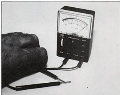
Always check calibration before using ohmmeter. Touch probes together, then turn calibration wheel until needle points to 0 ohms. This also checks the built-in battery.
