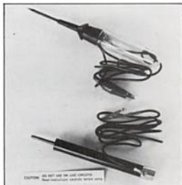
Two types of circuit test lamps. Top one indicates voltage in live circuits. Bottom one is battery-operated self-powered test lamp, used to check circuit continuity with power off. It's the one to use to check your harness as described in accompanying text. As package precaution says, do not use it on live circuits. Photo by Ron Sessions.
