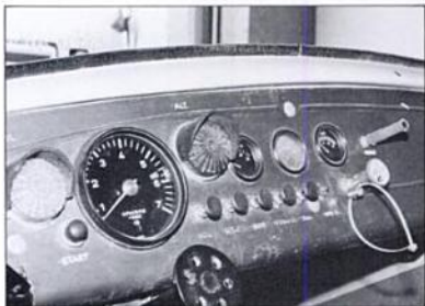
Trailer clearance lamps, shaded from sun, make hard-to-miss warning lamps on this competition Baja Bug. Stick at right of instrument panel is horn-switch actuator that can be operated with a slap of hand. Large knob below floods engine and driver's compartment with Halon-13 fire-extinguishing agent. Photo by Jeff Hibbard.
