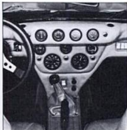
When I laid out instrument panel of my Bernardi component car, I made room for all instrumentation I wanted: nine gauges, five warning lamps and assorted switches. On the road, everything performs just the way I'd hoped.
