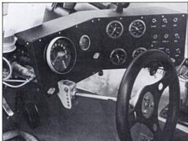
Race car's angled instrument panel provides optimum gauge visibility and switch access from driver's seat. Dzus 1/4-turn fasteners allow quick panel removal for pit repairs. Tach is positioned so red line is straight up. Photo by Tom Monroe.
