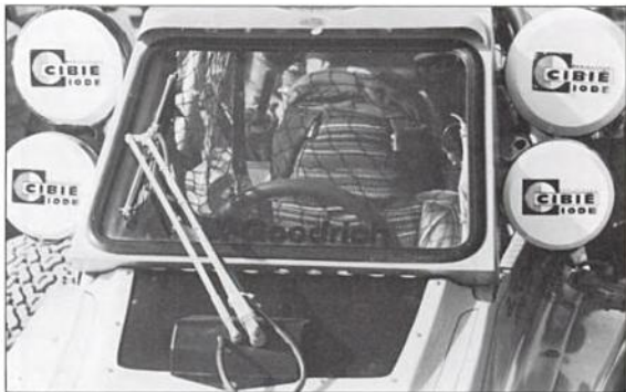
Original 6-volt system was barely adequate for stock pre-1967 VWs—no way would it handle this much candlepower on an off-road buggy! You'll probably want to replace 6-volt system anyway, because original system will probably be showing its age—and most aftermarket electrical accessories are 12 volt. Photo by Tom Monroe.
