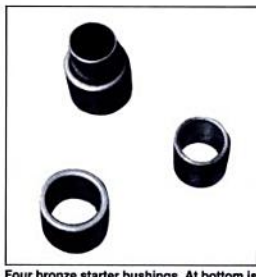
Four bronze starter bushings. At bottom is stock 6-volt bushing. Right one is stock 12-volt bushing. At top is stock 6-volt bushing and special sleeve inside it to neck down bushing ID when switching from 6-volt starter to 12-volt one.
