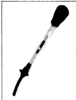
Hydrometer contains weighted float, which sits shallower or deeper in electrolyte sample, depending on specific gravity. Reading on float is taken at point where it protrudes from liquid.
