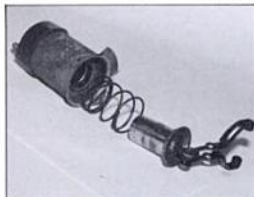
I took this GM starter solenoid apart so you could see the movable core clearly. Core is attached to forked lever to move drive gear when starter is operated.
