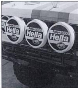
Lamps and electrical motors are the two major types of electrical loads found on cars. High-power driving lamps like these use a lot of juice, so battery and alternator (sources) and wires (paths) must be sized accordingly. Photo by Tom Monroe.
