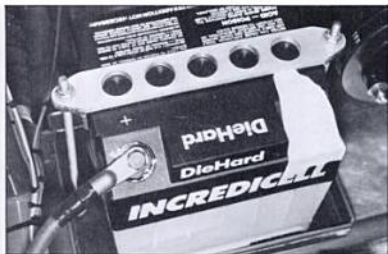
In his street legal sprint car, Ron Fournier located battery behind seat in tail of car, for improved weight distribution. This also placed battery within a few feet of rear-mounted alternator.
