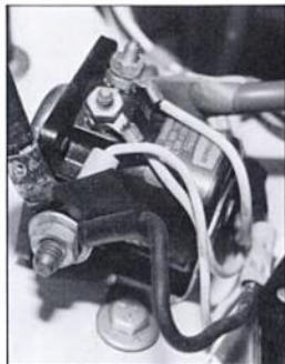
Typical Ford starter solenoid. Although it acts as a relay in the battery-to-starter cable, it contains a movable core, so is correctly called a solenoid.
