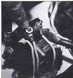
This is where other end of resistor bypass wire is attached. During engine cranking, full battery voltage is available at "I" terminal. If your car has an ignition resistor, use starter solenoid with bypass terminal—identical solenoids are made without "I" terminal.
