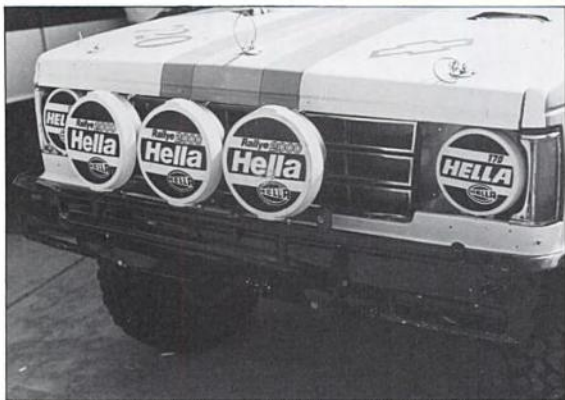
Lights are resistance loads. Headlamps and driving lamps on this Class 7 4X4 off-road racing truck are heavy loads that draw high current, so they deserve special consideration when selecting wire, circuit protection, battery and alternator. Photo by Tom Monroe.
