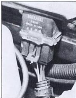
Newer cars rely on relays, such as this one, to operate computer-controlled emission devices. Computer's low-current circuitry operates low-current relay, which in turn operates high-current device.
