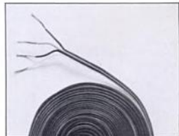
For easy routing, trailer wire in the four standard colors—green, yellow, brown and white—is sold "stuck together" like this. Individual wires can be pulled or slit apart, if done carefully. Photo by Jim Barrett.
