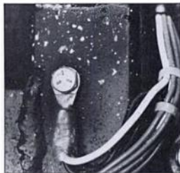
Ground stud or ground bolt is used to provide common grounding point for two or more components. Here, tailamps mounted on fiberglass car body are all grounded to car's metal frame at this one point.
