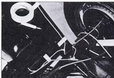
The clothesline is installed to represent final harness routing. Note how line is run inside chassis rail for added protection. Branch point leads to fuel-gauge sender. It must not interfere with movement of rear axle.
