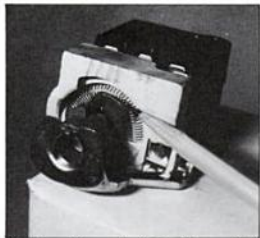
Coil of resistance wire in headlamp switch is a rheostat , used to control intensity of gauge illumination. Because resistance wire heats up during operation, it is installed in heatproof ceramic housing.
