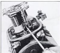
Mechanical voltage regulator controls current output of generator through set of movable points and calibrated coils. Current flows when points are touching. On one shown here, points are adjustable. For best performance, keep points clean. Photo by Ron Sessions.
