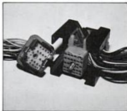
Fuse panel and main wiring harness from my Pinto donor car. Panel mounts under dash. Engine harness (left) passes through bulkhead and plugs into back of panel.
