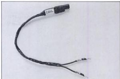
Coil lead made by race car electrician Frank Parker is example of good race-car wiring. He prefers harness wrap of nonadhesive loom tape to protect wires from dirt and grime. All leads are clearly marked with indelible ink on waterproof wrap-around labels for quick reference by pit crew during race. Aircraft-grade seamless ring terminals are used on coil leads. Photo by Jim Barrett.
