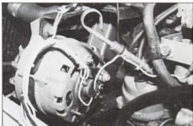
Nylon ties are used to retain electric choke feed wire to oil dipstick tube. It's better to use any available support rather than fabricating additional parts. Note slight amount of slack in generator wires to permit adjustment of drive belt.
