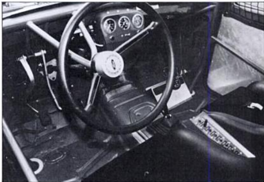
Class 7 off-road racing truck relies on minimum instrumentation, resulting in simple, uncluttered dash. Light switches are mounted on panel between seats. Photo by Tom Monroe.
