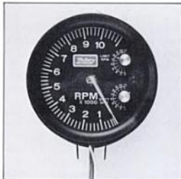
Race drivers usually dispense with speed in favor of large, accurate tach with rev limiter. Shown here is the RPM Limiting Pro Tach from Mallory Ignition. It also has shift-point indicator lamp, set by dial at bottom right. Photo by Jim Barrett.
