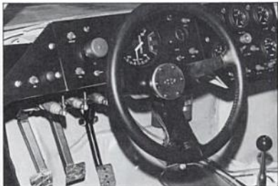
Off-road racers prefer widely spaced switches—less chance of driver hitting wrong switch while bouncing over rough terrain. Photo by Tom Monroe.
