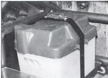
Battery box must be securely fastened to be effective. Photo by Jeff Hibbard.
