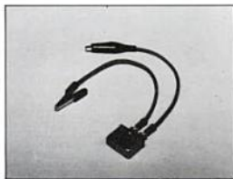
You can use a jumper wire like this to bypass controls when testing a circuit—never bypass a load. Note auto-reset circuit breaker I installed as a precaution. I sometimes use this wire to extend one of my ohmmeter leads when doing continuity checking.
