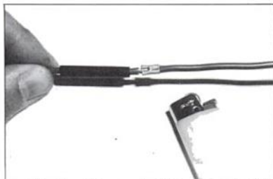
If you intend to shrink wrap a butt joint, use a non-insulated terminal.
