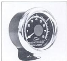
Tach reads revolutions per minute (rpm). Sun Super Tach II, model CP7901, has adjustable "red line" to indicate optimum shift points. Photo courtesy of Pentron Products Inc.
