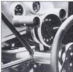
Race drivers also depend on large indicator lamps that quickly grab attention. These Pro-Lites from Auto Meter indicate low oil and fuel pressure; here, they're mounted on tach for best visibility. Photo courtesy of Auto Meter.
