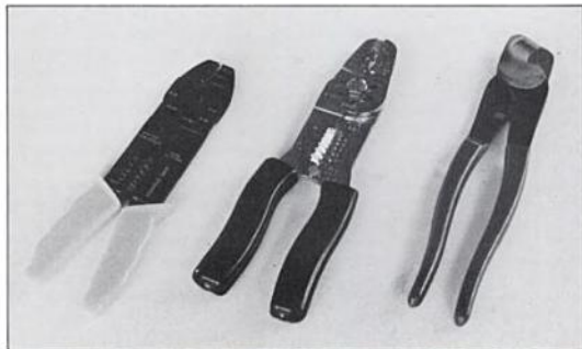
Tools required for installing terminals include a wire cutter, stripper and crimper. Two tools on left do all three. Photo by Ron Sessions.
