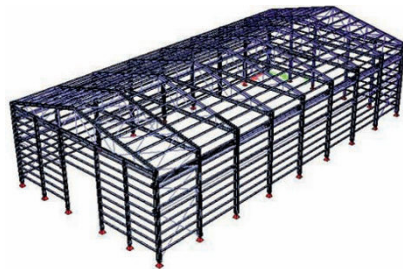
Fig. 2.1. Model for a single story industrial building
