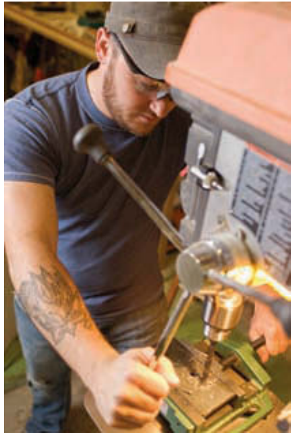
Figure 4-8 Drill presses used in the home shop are usually operated manually.
