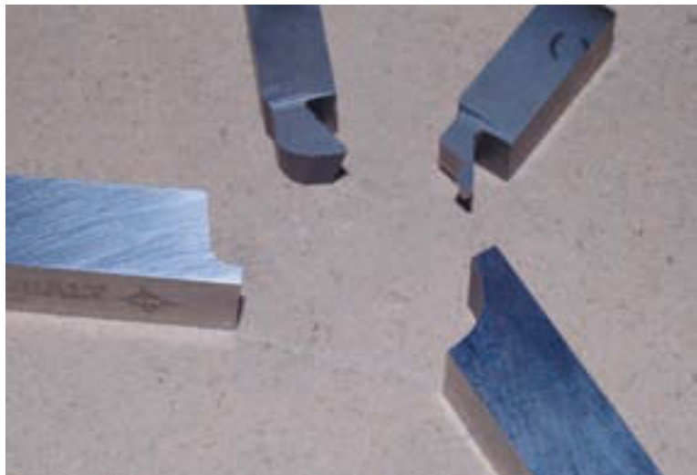
Figure 5-10 Here is a collection of special tool bit profiles.
