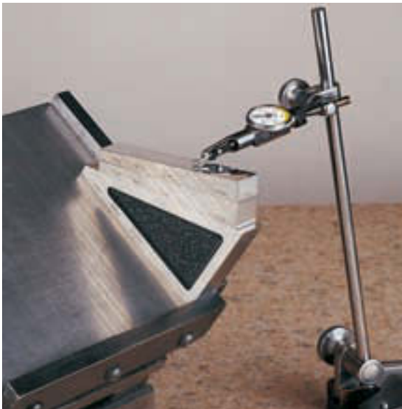
Figure 2-29 Dial test indicators serve a variety of uses in the machine shop. Here an indicator is used with a surface gage.
