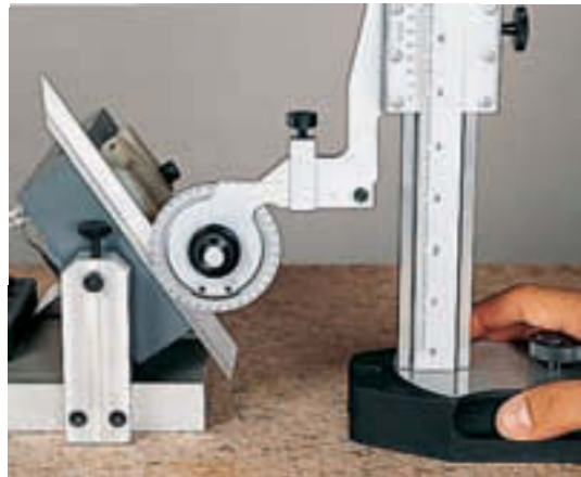
Figure 2-18 A vernier bevel protractor used in combination with a height gage.
