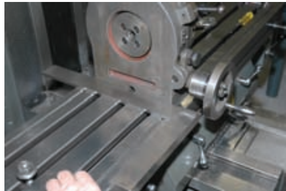
Photo 13 Squaring the rotary table to the milling machine table.
