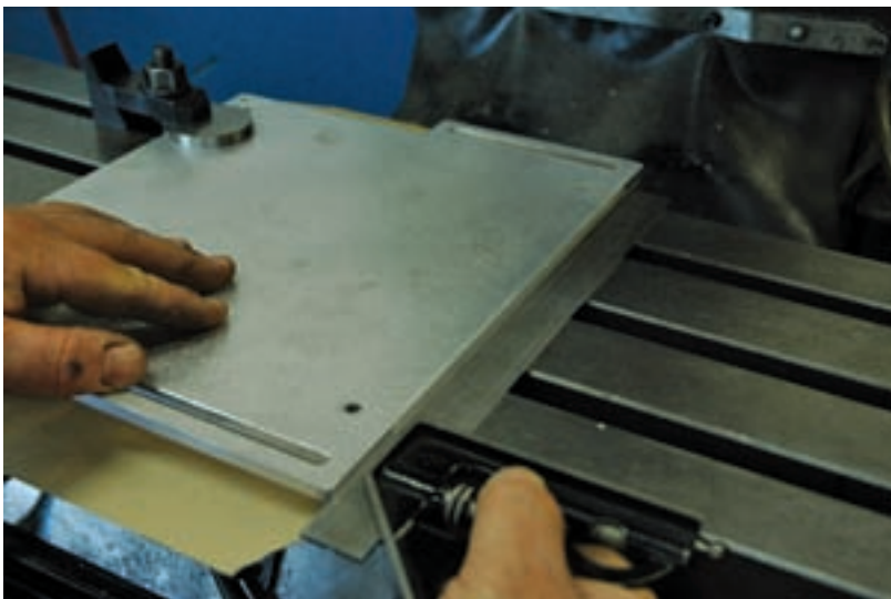
Figure 7-8 The workpiece is aligned using a combination square.
