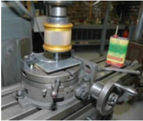
Photo 6 Machining the bore.
