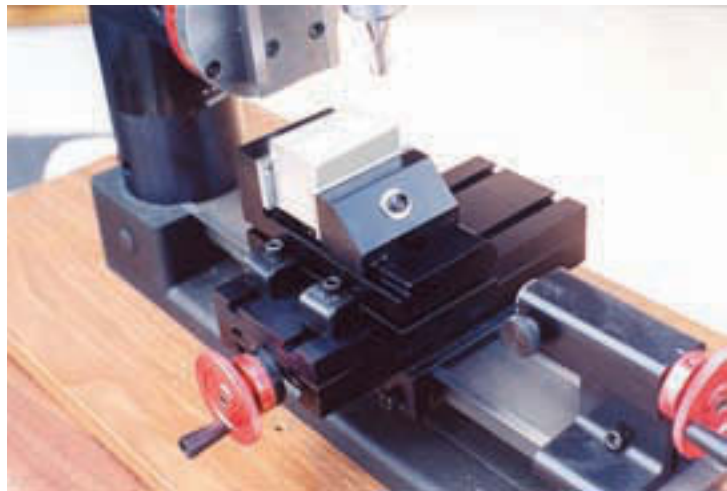
Figure 3-6 Drill, or mill, vises have smooth jaws and are often sold as accessories by mill manufacturers.
