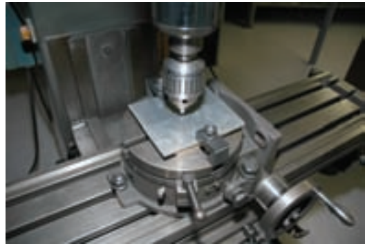
Photo 4 Setting up to make the sample part. The spindle is aligned with the "X" on the work piece.
