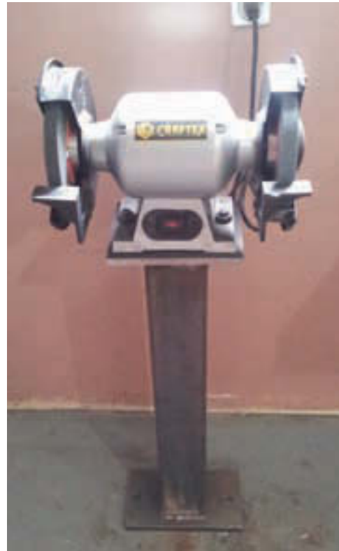
Photo 1 An eight-inch bench grinder mounted on a pedestal.
