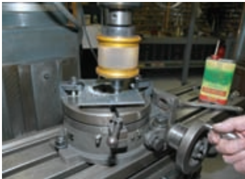
Photo 7 Finishing the bore by climb milling the last few thousandths of an inch.
