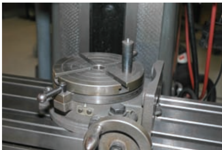
Photo 1 My rotary table. The plug setting on top is a centering plug made from the Morse shank of a drill bit.
