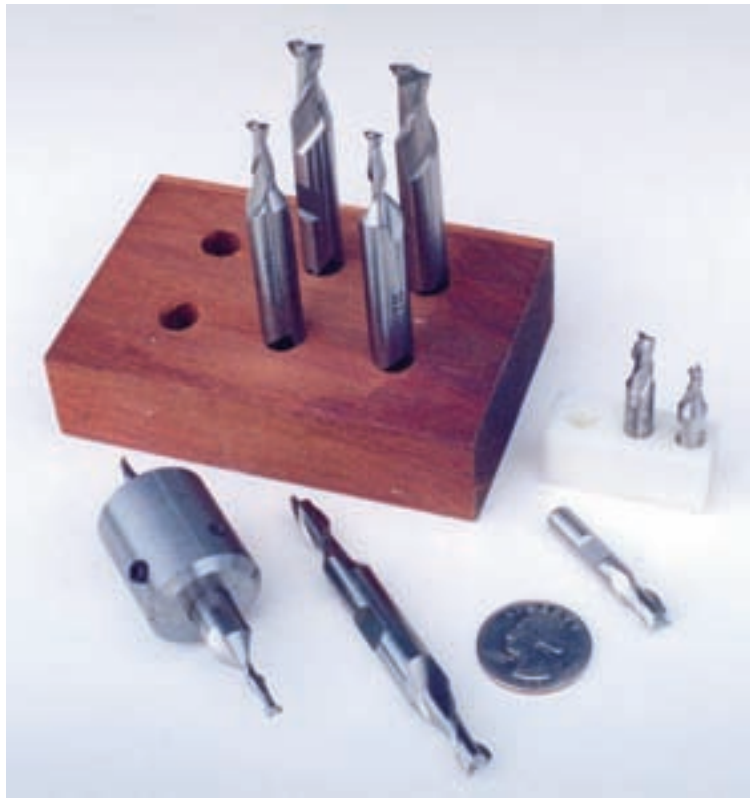
Figure 7-5 Shown is a set of end mills designed for a small bench-top mill.
