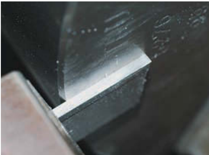
Figure 5-4 Cutting tools made of high-speed steel can be sharpened repeatedly. This is a parting, or cut-off tool.
