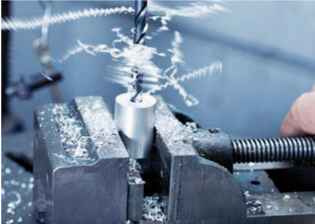
Figure 4-7 A drill press vise holds a workpiece during drilling.
