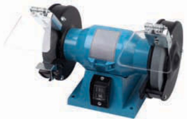
Figure 1-11 A benchtop grinding wheel. Note the safety shields in front of each wheel.
