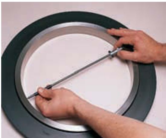
Figure 2-23 Taking a measurement with an inside micrometer.
