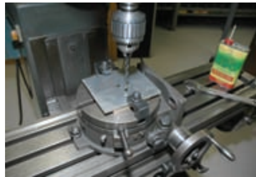
Photo 5 Drilling a hole to begin milling the center bore.
