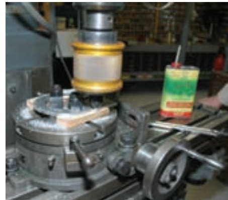
Photo 10 Finishing the outer radius.
