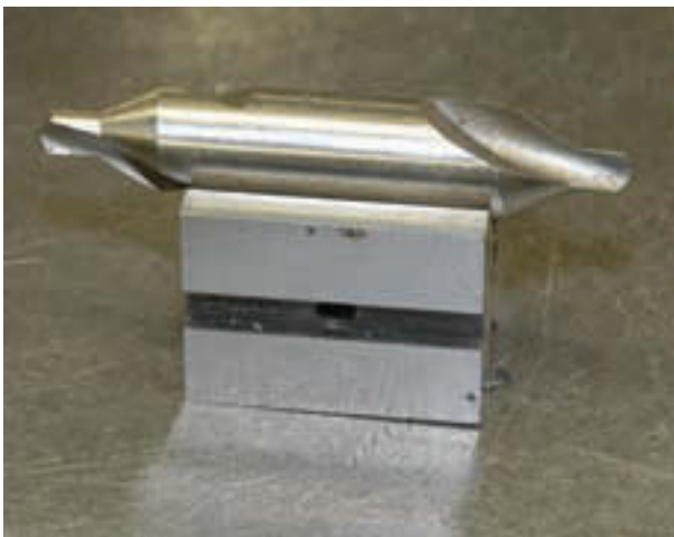
Photo 1 A combination drill and countersink used for machining centers in a part.
