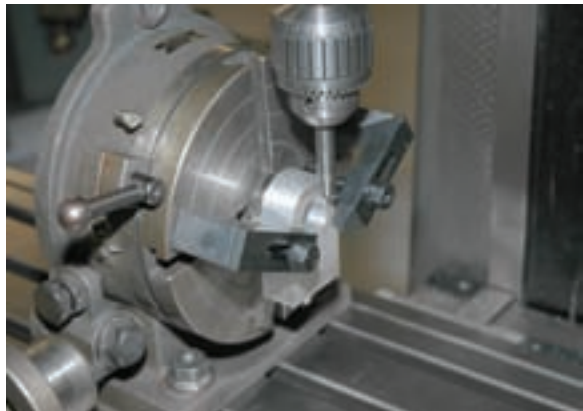
Photo 15 Locating the spindle axis relative to the X-axis of the part.
