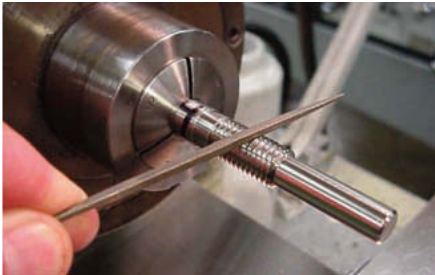
Figure 6-25 A triangular file cleans up a damaged thread.
