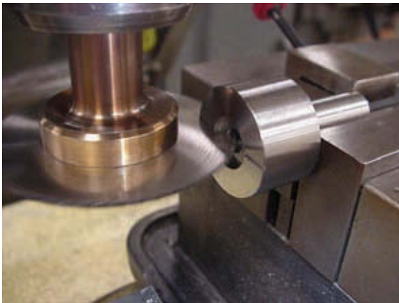
Figure 7-2 Here is an example of a slitting saw make a cut on the face of a part.
