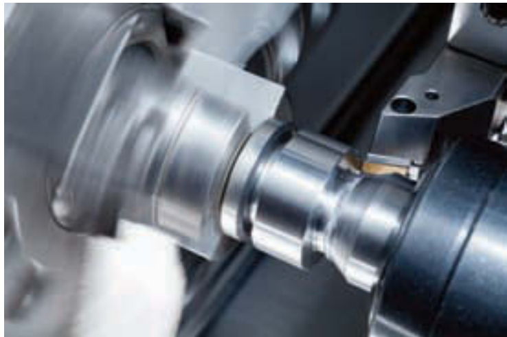
Figure 1-1 An example of a machine tool creating a cylindrical shape from a metal bar.
