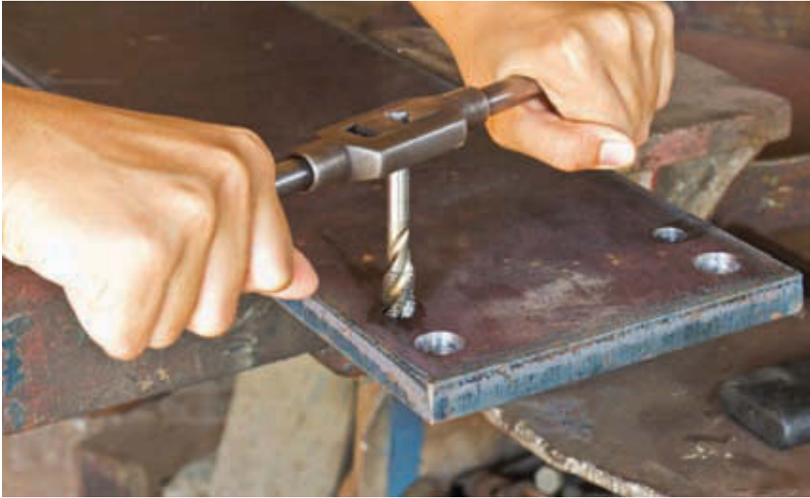
Figure 4-18 Threads being produced by a manual tap.
