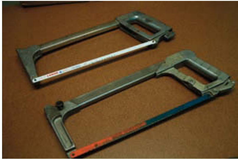
Figure 3-8 Use a hacksaw to cut metal down to a manageable size before machining.
