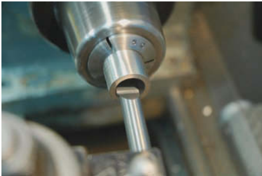
Figure 6-18. Here's an example of a boring tool cutting tapers in a workpiece.
