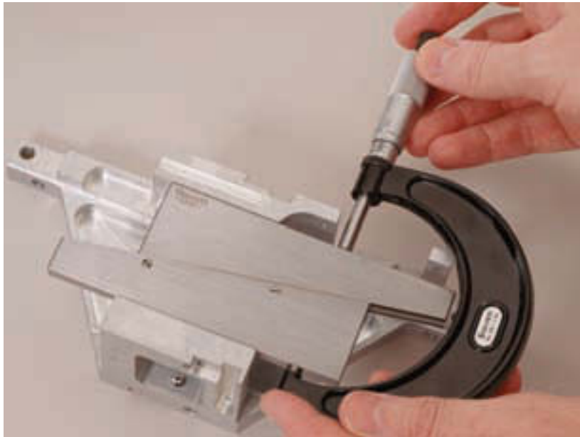
Figure 2-32 Measuring the width of a slot using adjustable parallels and a micrometer.
