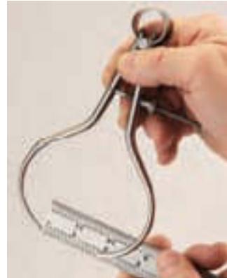
Figure 2-1 In some cases, more than one tool is needed. Here a caliper is used with a steel rule to take a measurement.
