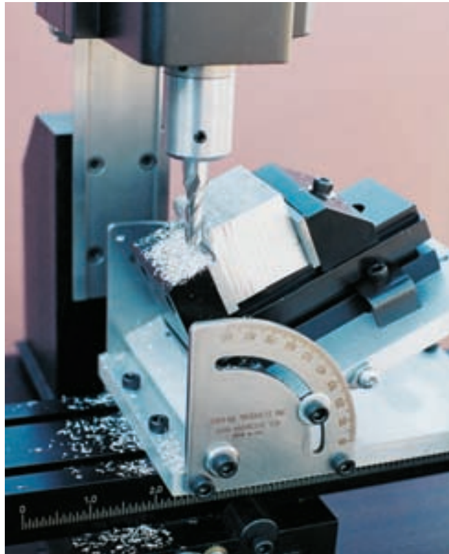
Figure 7-10 Mill vises are often used to hold work in place. The one shown here is clamped to a tilting table. Note the protractor to align the table to the proper angle.
