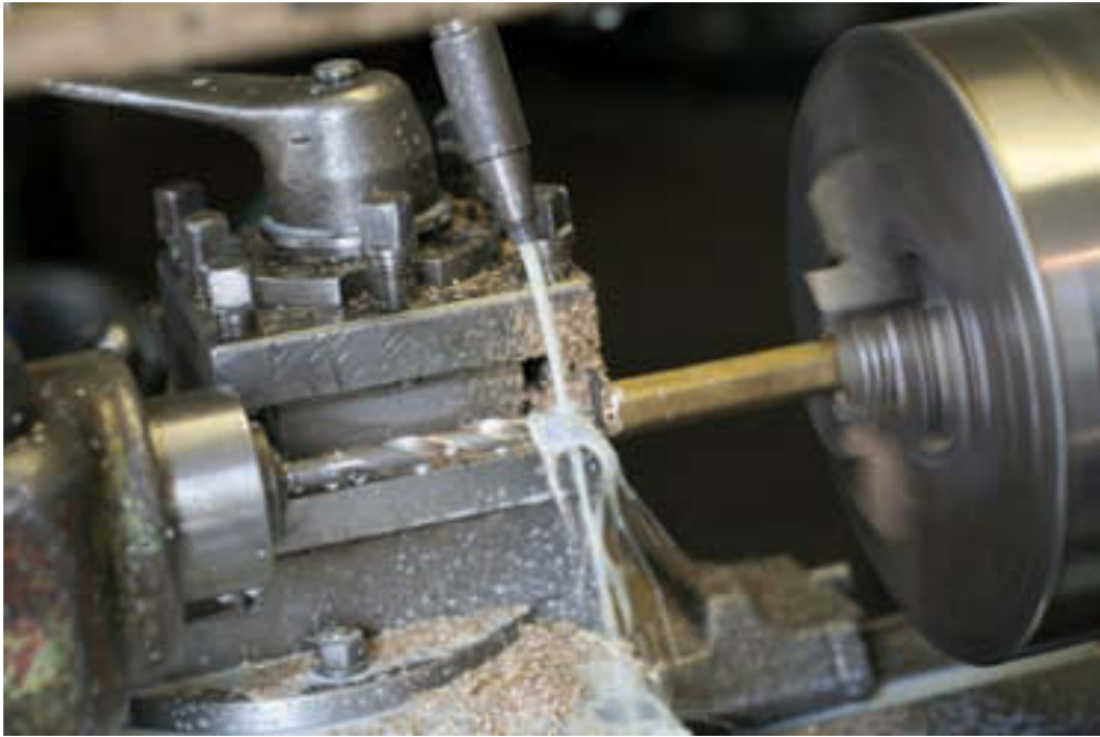
Figure 5-11 Cutting fluid applied to a workpiece.
