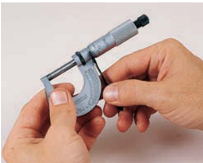
Figure 2-27 Adjusting for a zero reading with a spanner wrench supplied by the tool manufacturer.
