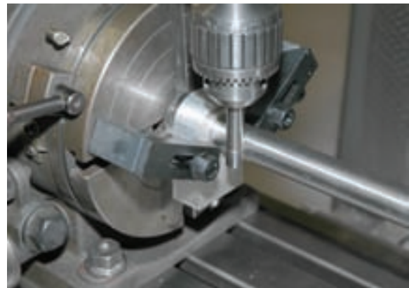
Photo 14 Locating the center of the rotary table relative to the spindle axis.
