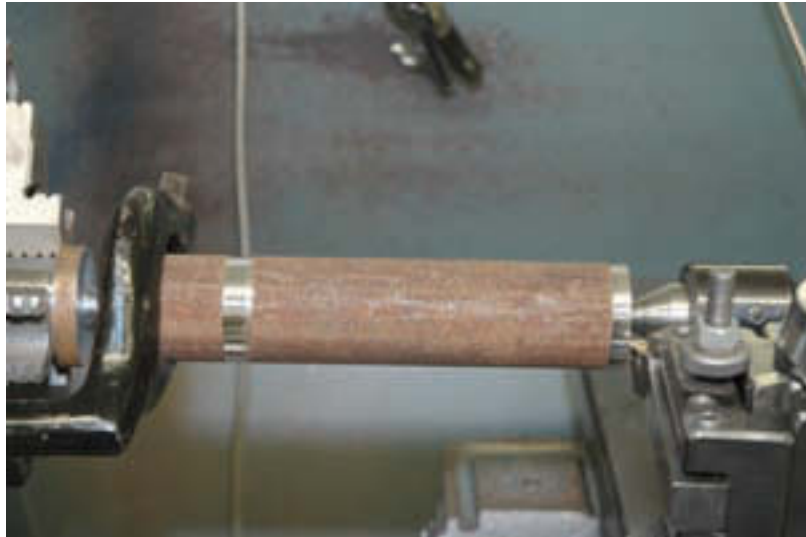
Photo 8 Test cuts to determine the amount of taper — if any.
