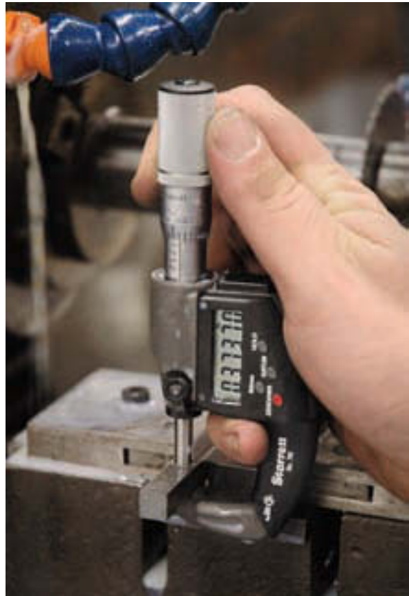
Figure 2-22 Micrometer with an electronic readout.
