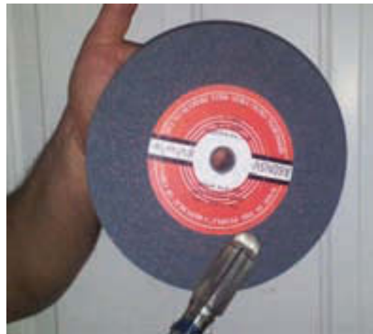
Photo 3 Tap the wheel with plastic or wood to check for flaws.
