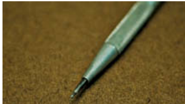
Figure 3-1 Scribers allow the machinist to etch layout lines directly on the metal.
