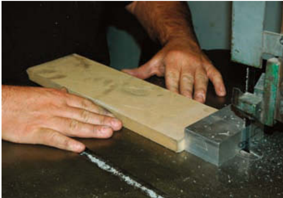
Figure 3-11 A push stick, or in this case a “belly board,” keeps the operator’s hands away from the moving blade.
