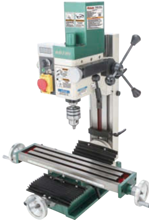
Figure 1-7 A vertical benchtop mill.
