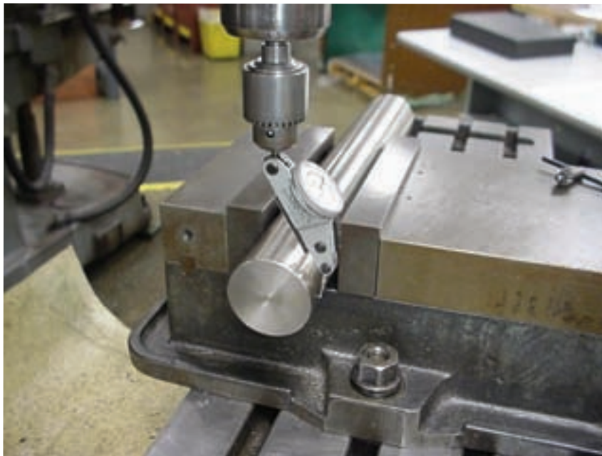
Figure 7-11 Use a dial indicator to position work accurately.
