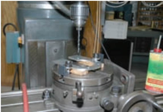
Photo 11 Drilling the bolt hole pattern.
