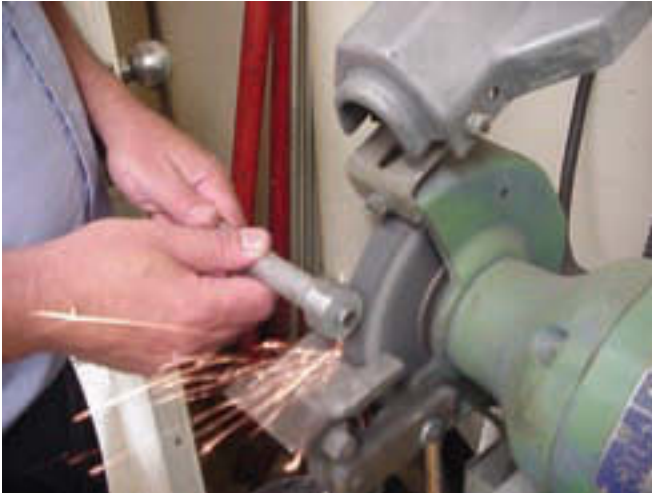
Figure 3-13 Here is an example of dressing the wheel on a pedestal grinder.
