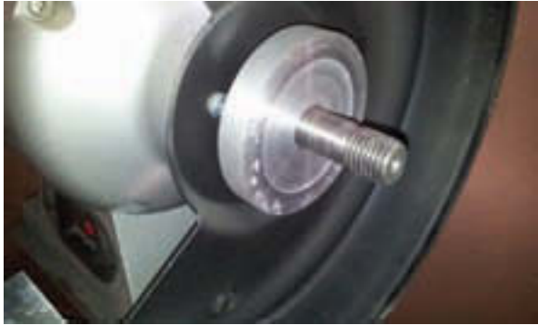
Photo 6 A homemade clamping washer to replace the stamped original.
