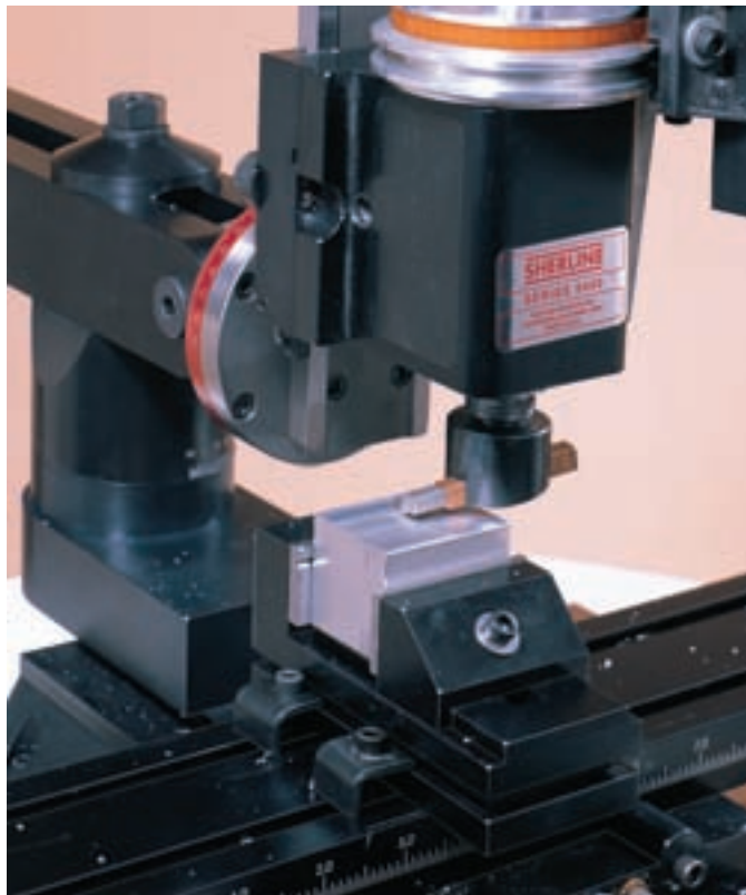
Figure 7-6 A fly cutter, such as the one shown, is capable of producing a smooth finish.
