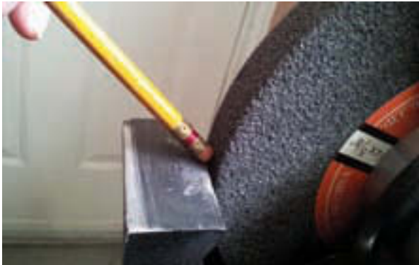
Photo 4 Checking clearance with a pencil.
