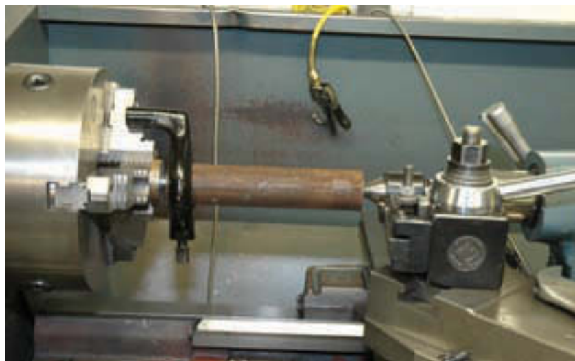
Photo 7 A part set up between centers.
