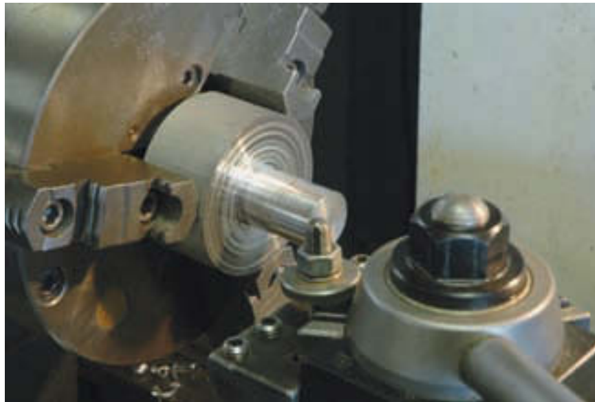
Figure 6-8 A three-jaw chuck provides a quick way to setup work on a lathe.
