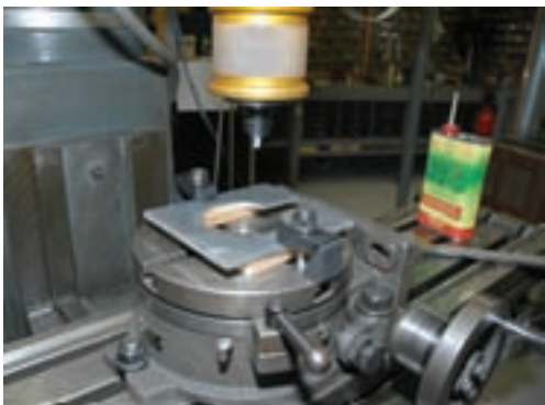
Photo 8 Finished bore and slot.
