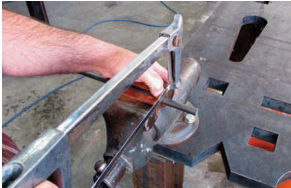
Figure 3-9 Use your thumb as a guide to create a starter notch in the metal.
