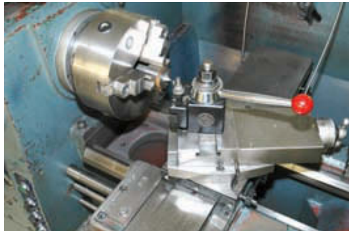
Photo 4 Setup for machining a 60-degree center.
