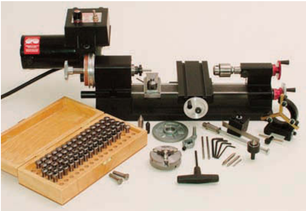
Figure 6-12 The box in the foreground holds a collection of collets. To keep the workpiece aligned properly, choose the correct size collet.
