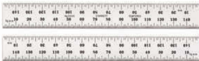
Figure 2-3 Steel rule with metric graduations.
