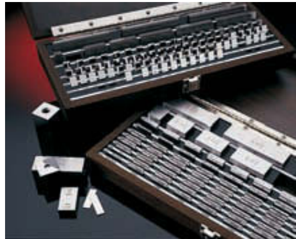
Figure 2-30 Among other uses, precision gage blocks help calibrate machine shop tools.
