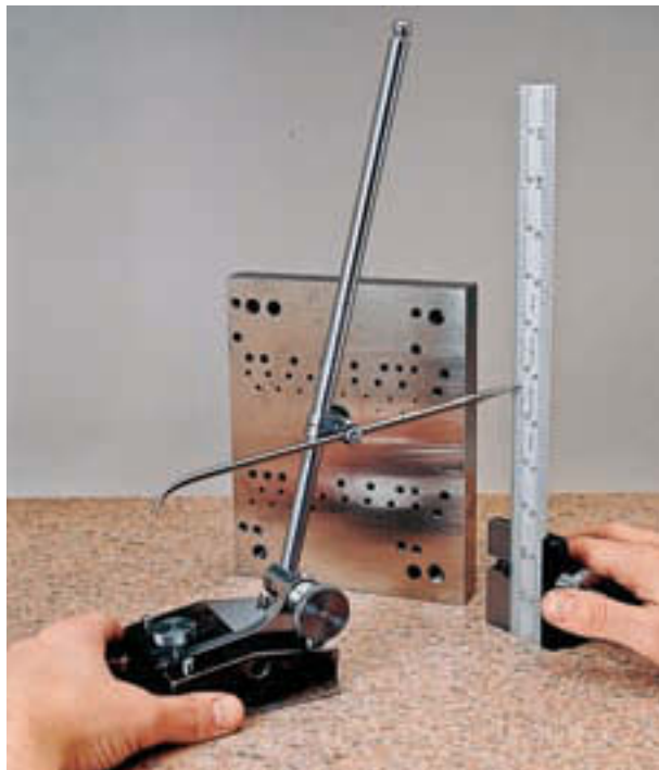
Figure 2-31 Surface gages are used to transfer measurements.
