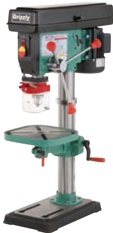
Figure 4-1 This is a typical bench-top drill press for home shop use.
