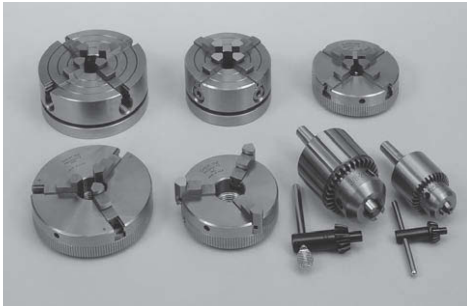
Figure 5-3 Here is a collection of drill chucks and three- and four-jaw chucks.
