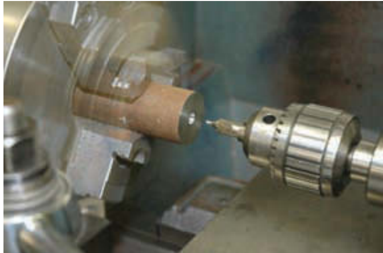
Photo 2 Drilling the center hole in one end of the material.
