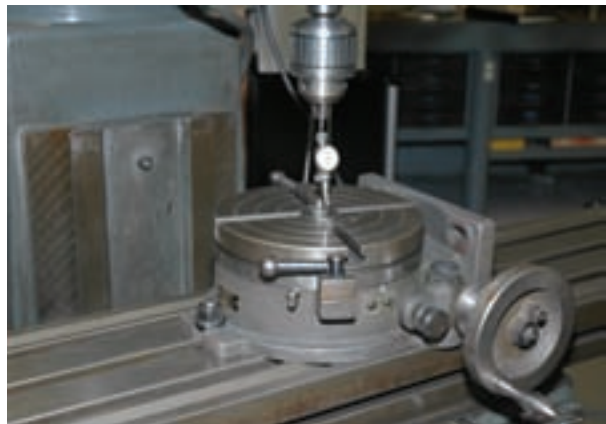
Photo 2 Locating the center of the rotary table relative to the axis of the milling machine spindle.
