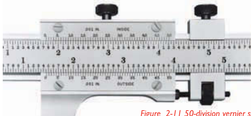
Figure 2-11 50-division vernier scale.
