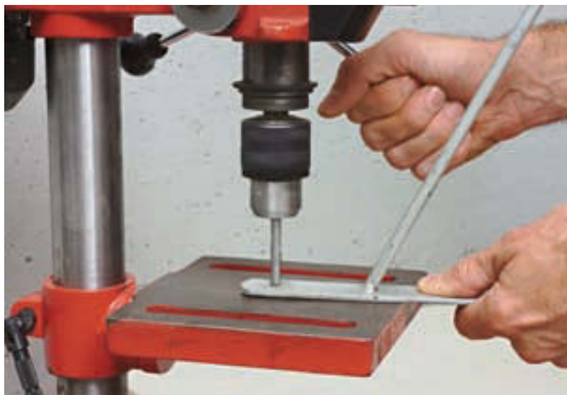
Figure 4-4 Here's an example where the work can be safely held in place without the use of clamps.
