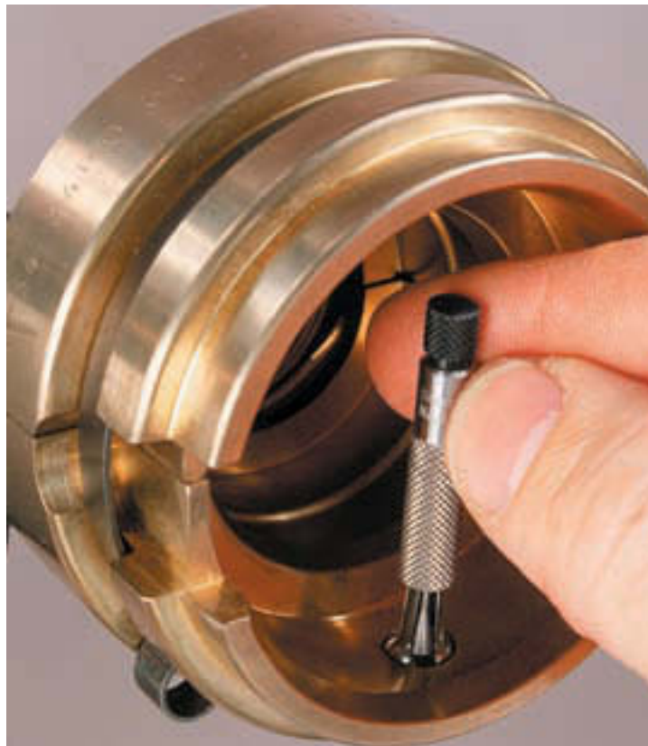
Figure 2-4 Small-hole gages are used to measure hole diameters.
