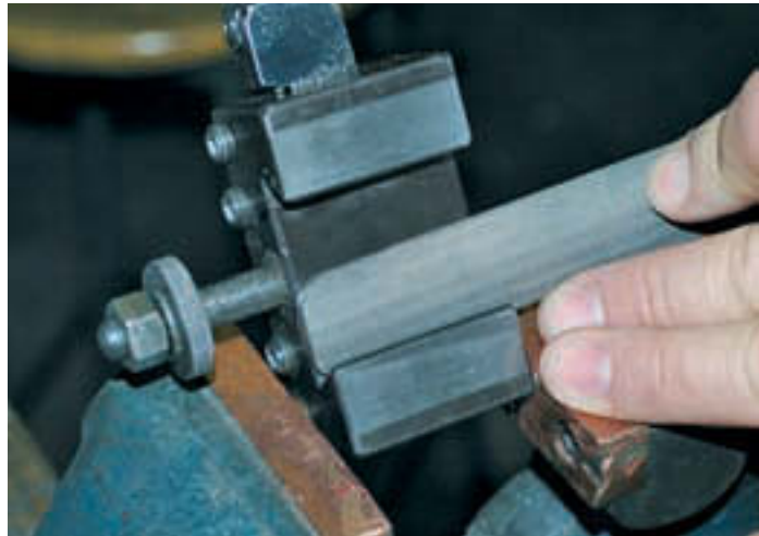
Figure 3-4 Here is a single-cut file smoothing a part.
