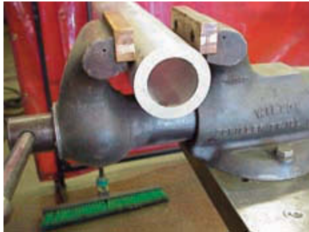
Figure 3-7 Clamp round work below the tops of the jaws to hold it steady.
