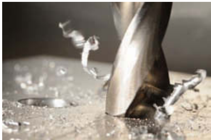
Figure I-3 A drill boring into a metal surface.
