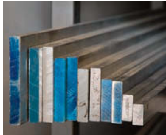
Figure 3-14 Store flats on edge to save space. The owner of this shop used a color coding system to identify materials.
