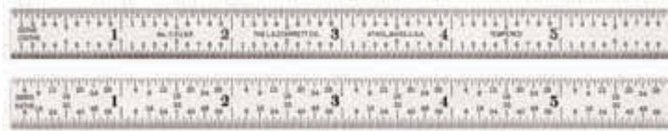
Figure 2-2 (Upper view) Steel rule with decimal inch graduations; (Lower view) Steel rule with fractional inch graduations.
