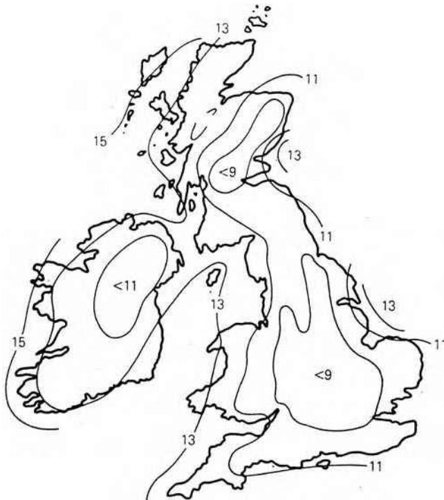
FIGURE 3.21 Isovent map of the U.K. in knots at open sites, excluding hilltops. (From Freris, L.L., Wind Energy Conversion Systems , Prentice Hall, London, 1990.)
