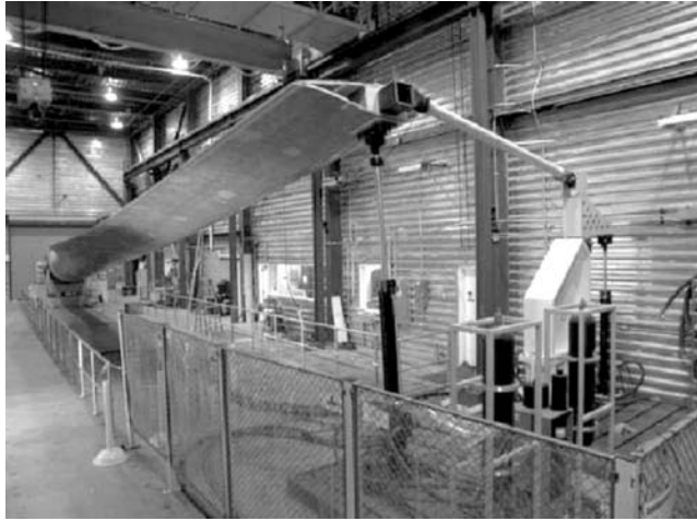
Figure 7.13 NREL's dual-axis forced displacement test set-up (White, 2004)
