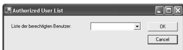
Figure 6.5 String expansion taken into account
