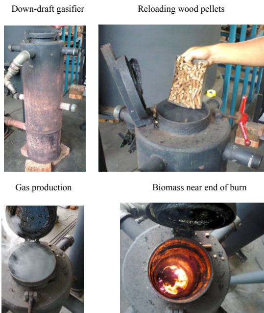
Figure 8. USM's 5 kW down-draft wood pellet gasifier.
