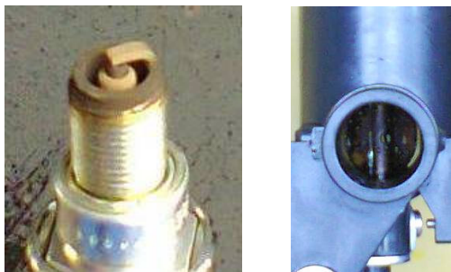
Figure 14. Spark plug at 2 hours of operation (left) and fuel valve after 3.5 hours (right).
