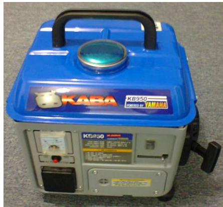
Figure 2. The Yamaha 950, 650 W genset, assembled by Kaba.
