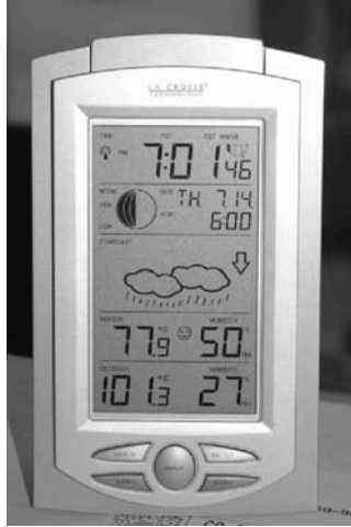
FIGURE 4.8 July 14, 2005. Summertime comfortable temperature spread of 23.4^{\circ} maintained without mechanical cooling. (Author's photo.)
