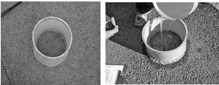
FIGURE 7.4 Infiltration rate testing of in-place pervious concrete. (From ASTM C1701-09.)
