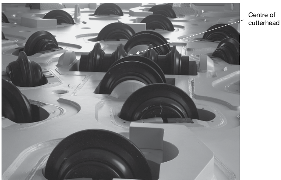
Figure 5.23 An example of some hard rock disc cutters (as used in granite). Note the arrangement of the cutters from the centre of the cutterhead to the edge to ensure all the face is excavated. (Courtesy of Herrenknecht.)
