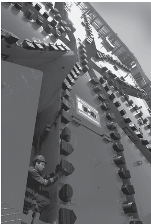
Figure 5.25 Cutter dressing used on a Mixshield TBM in Shanghai through sand, clay and loose gravel/boulders. (Courtesy of Herrenknecht.)
