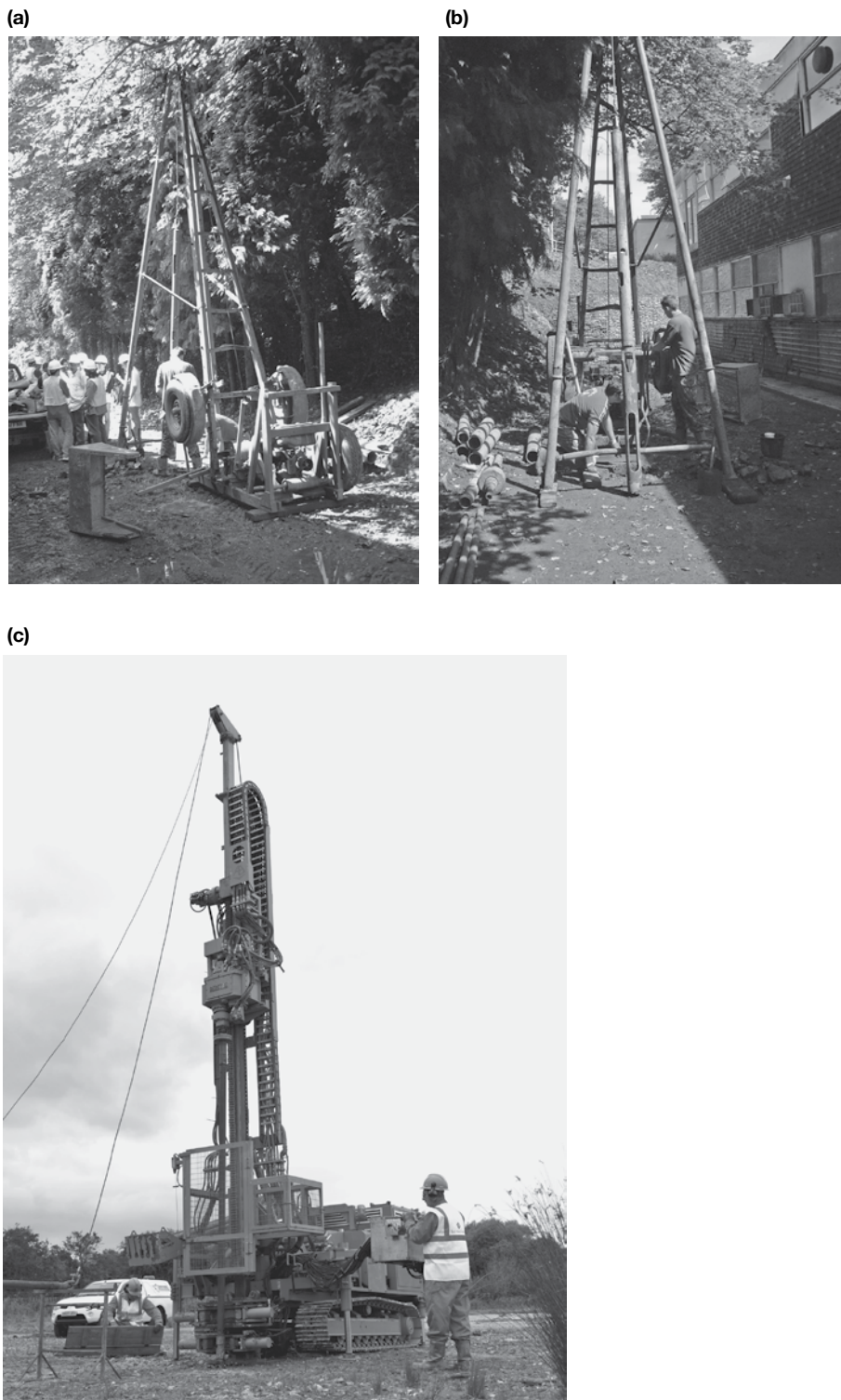
Figure 2.4 (a) and (b) Cable percussion rig and (c) rotary drilling rig. (Courtesy of Soil Mechanics.)
