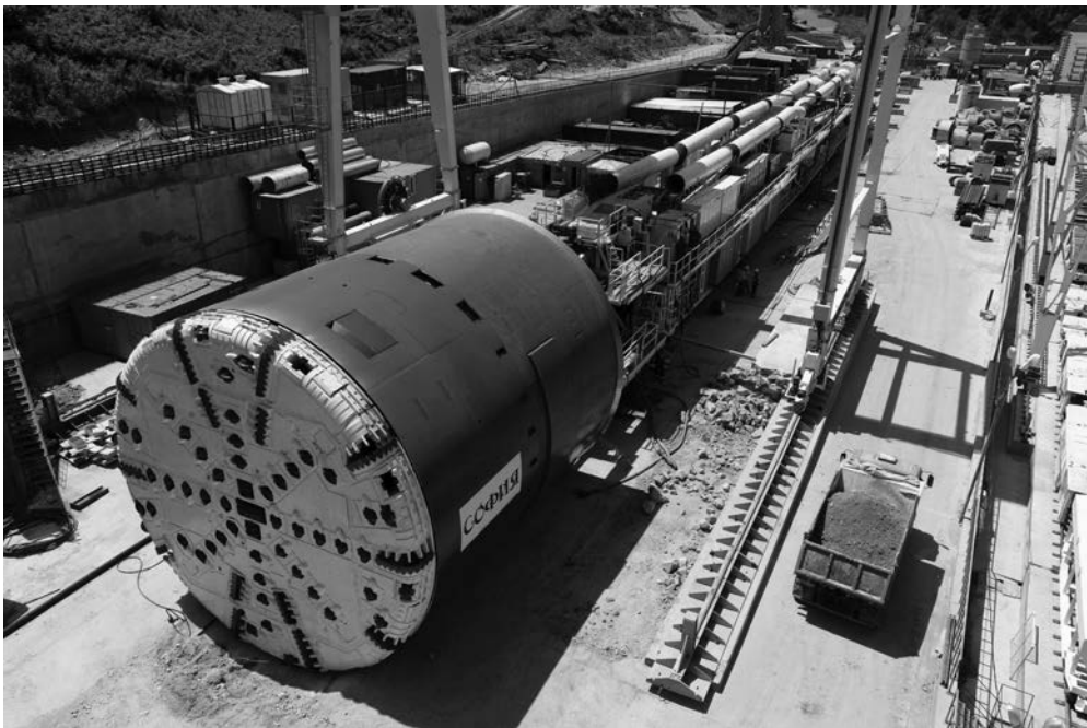
Figure 8.55 A 10.0 m diameter double-shield TBM used in Sochi, Russia. (Courtesy of The Robbins Company.)
