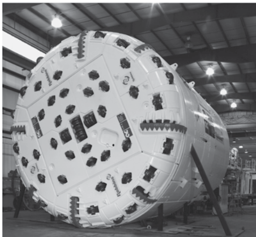
Figure 5.20 Single-shield TBM used in Laos (7.6 m diameter, 5.5 km length, variable ground consisting of sandstone, siltstone and mudstone). (Courtesy of The Robbins Company.)
