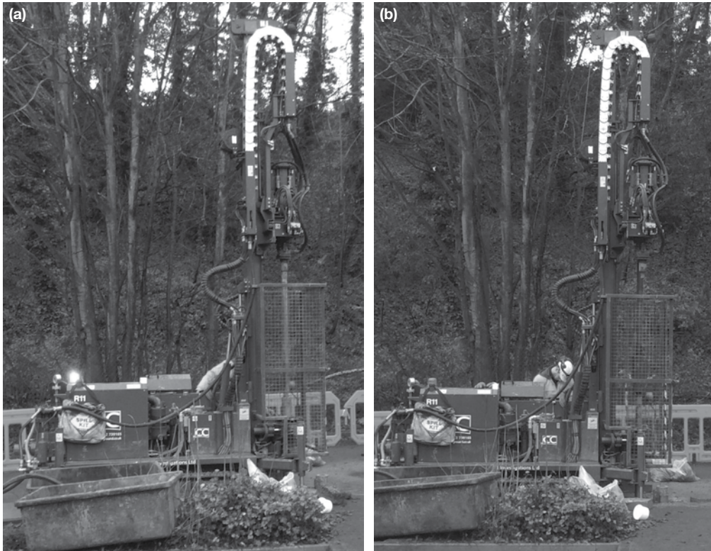
Figure 2.5 Dual mast drilling rig. (a) one mast can be used for conducting rotary drilling operations and (b) the other mast can conduct Standard Penetration Tests.
