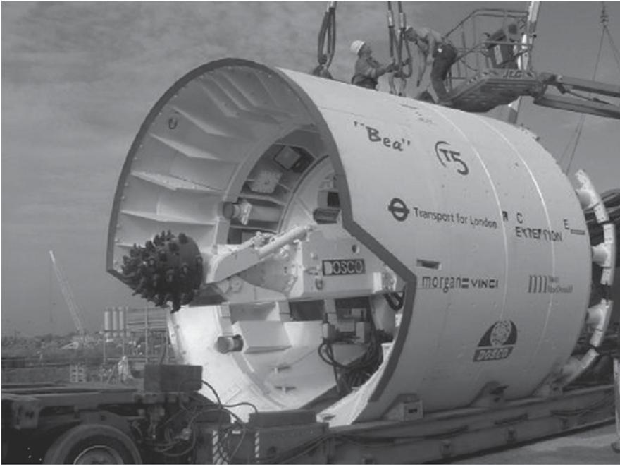
Figure 5.8 Refurbished Dosco boom-in-shield tunnelling machine as used for constructing the Piccadilly Line Extension (PiccEx) Tunnel to Heathrow Terminal 5 in the United Kingdom.
