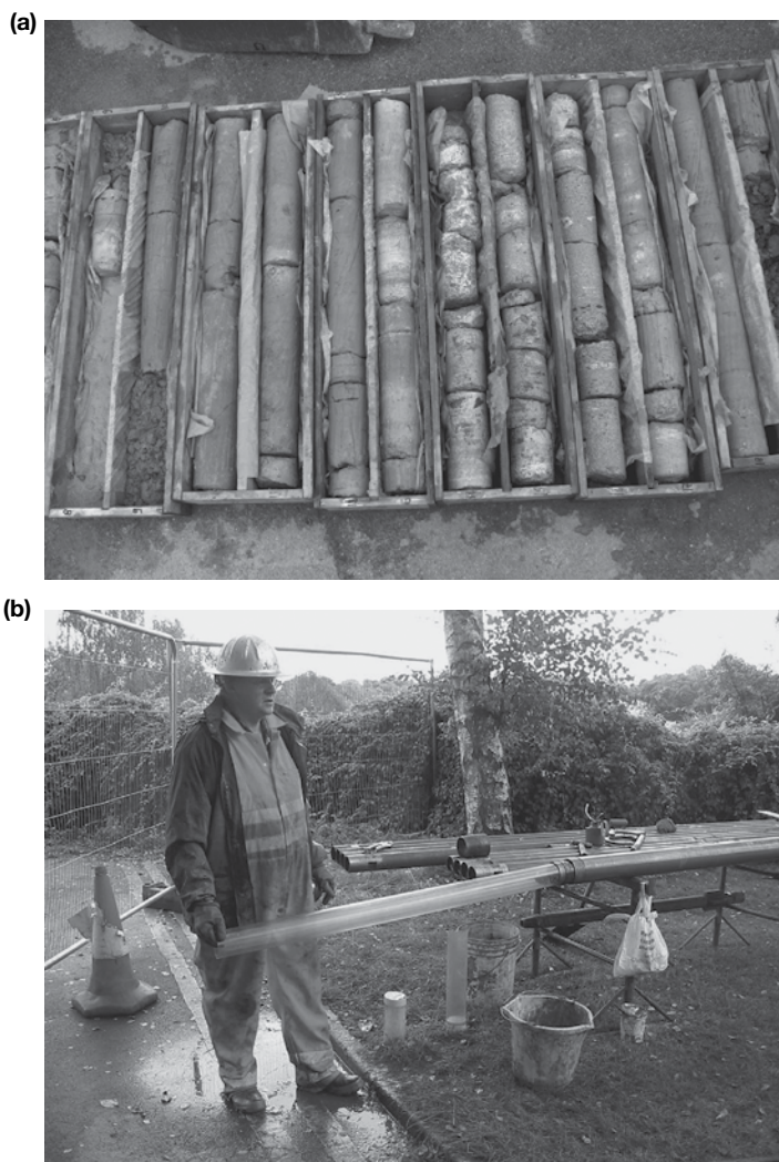
Figure 2.6 (a) Example of continuous rock cores obtained from rotary drilling and (b) triple core barrel sampler (double core barrel with a plastic liner) used with rotary drilling.
