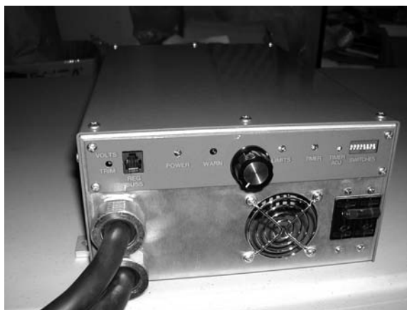
FIGURE 9-4 The Manzita Micro PFC-20, an extremely versatile battery charger.
