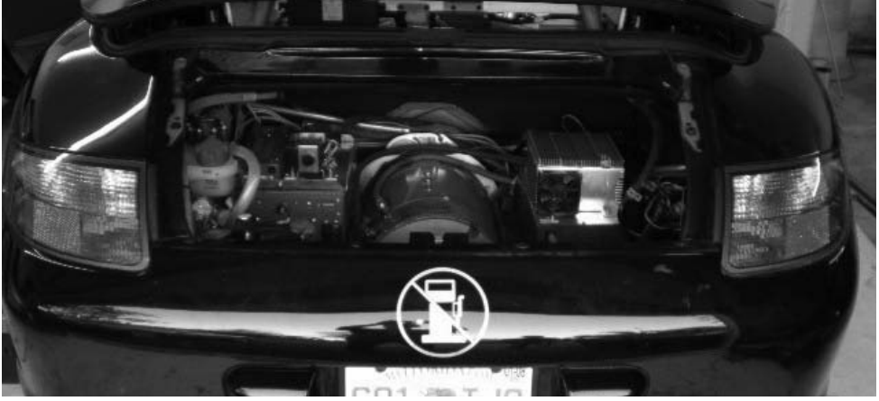
FIGURE 10-19 Porsche electric motor power cabling in the trunk.
