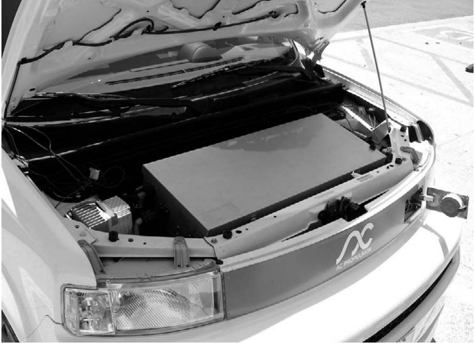
FIGURE 7-9 AC Propulsion 120kW power electronics drivetrain in the eBox.
