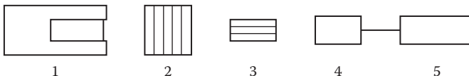
FIGURE 2.66 Block diagram of LAC meter: (1) Source and collimator of \gamma -radiation, (2) absorber, (3) collimator, (4) scintillator, (5) analyzer. (Reprinted from Yu. Potapov, Yu. Borisov, V. Chmyhiv, and D. Beilin, “Research of Polymer Concrete Based on Low Molecular Polybutadiene, Part VIII: Chemical Resistance of Polymer Concrete,” J. Scientific Israel Technological Advantages 7, nos. 1–2 (2005): 72–78. With permission.)
