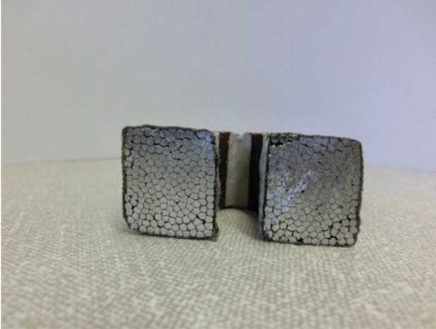
Figure 4.1 Pressed coil for high slot fill factor.
