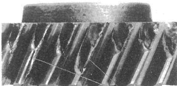
Fatigue failure from progressive pitting
