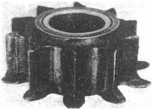
Spur gear virtually destroyed by foreign matter in the oil
