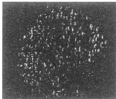
Metal transfer from a copper-coated steel ball loaded against steel plate \times 38 (courtesy K. L. Johnson)
