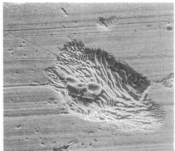
Corrosion of a cast iron bore
