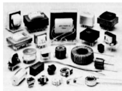
FIGURE 7.5-2 Elements with inductances arranged in various forms of coils.
