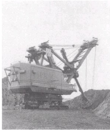
Bucyrus-Erie's "Big Brutus" mine shovel takes a 90-cubic-yard ( 69 \text{ m}^3 ) bite of Kansas coal.
