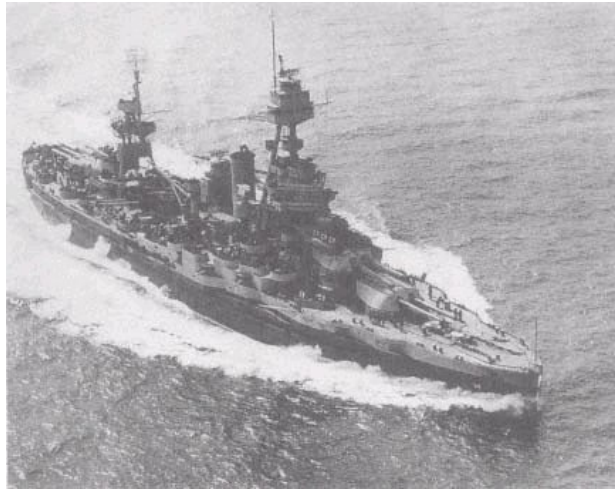
USS Texas, following modernization in 1925. The protected cruiser sports new tripod masts and hull armor for torpedo protection. Launched in 1912, the Texas was among the last U.S. dread-noughts to be powered by reciprocating engines.
