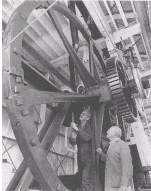
Power House Museum staff inspect the 14 foot flywheel of the Boulton & Watt rotative steam engine. Courtesy Museum of Applied Arts and Sciences.
