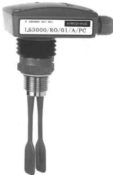
FIGURE 18.15 Design of a vibrating LS. The switch reacts to product viscosity changes, which dampens the vibration of the paddles. (From Messtechnik, K., Technical Data Sheets of Level Measurement Products , Krohne, Duisburg, Germany, 1996.)
