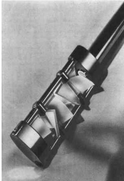
FIGURE 54.4 The rotor assembly of a dual-rotor, insertion axial turbine flowmeter for water flow measurement. This patented design renders the flowmeter insensitive to errors due to flow swirl; an important source of potential error in single-rotor axial turbine flowmeters. The rotations are sensed by two separate, electric impedance sensors. (Courtesy of Onicon Incorporated.)
