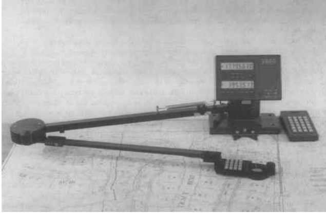
FIGURE 19.9 Arm digitizer lets one measure area, length, and coordinates and transmits the displayed data to a computer; it requires minimum desk space.
