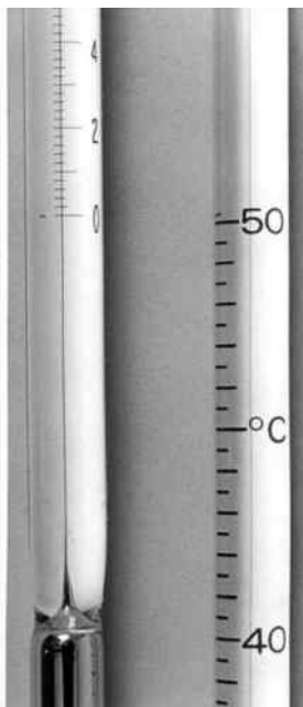
FIGURE 74.2 Good-quality thermometer (left) and general-purpose thermometer (right) showing the difference in the quality of scale markings. In the good-quality thermometer, the 0 °C pointing mark is immediately alongside the corresponding scale mark. In the general-purpose thermometer, the 50 °C pointing mark is about \frac{1}{4} scale divisions above the scale mark.
