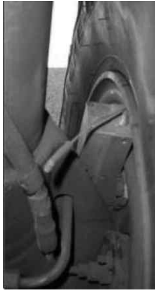
FIGURE 87.2 Ruggedized wireless wheel vibration and temperature sensor. (Courtesy of Solidica, Inc., Ann Arbor, MI.)
