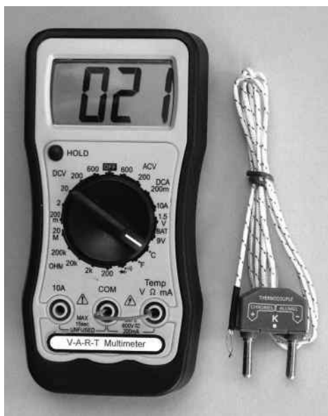
FIGURE 70.1 The simplest thermocouple thermometer. Inexpensive multimeters with a thermocouple temperature sensor obscure the need for detailed understanding of the principles of thermoelectricity for modern thermometry circuits. (Note shorted input and unplugged thermocouple. See Section 70.10.3.6.)
