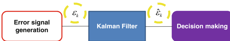
Fig. 4.4 Insertion of a Kalman filter in the monitoring system
