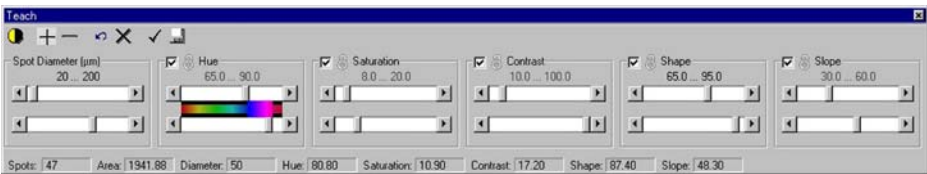
Fig. 3. Example for a spot teacher. Spots in the well image will be selected by simple mouse clicks to adapt the sliders to their values.
