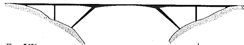
Figure 7.126 Suitable topography for inclined-leg frame bridges
