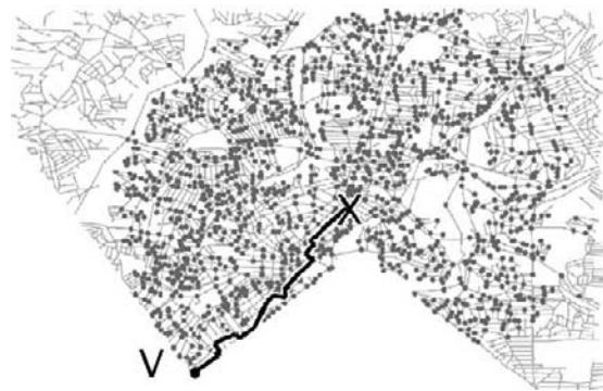
Figure 4.9 A map of Silver Spring, Maryland, and the vertices, highlighted by circles, that are visited when applying Dijkstra's algorithm in determining the shortest path from the vertex marked by X to the vertex marked by V.
