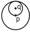
Figure 4.15 Example illustrating a nearest neighbor searching principle that given objects p and q and the distance d(q, p) between them, the distance from p of q 's nearest neighbor o cannot be greater than 2d(q, p) .
