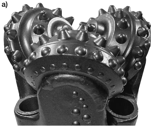
Figure 5.86 a) Rock drill bit and b) rock pre-reamer (courtesy of Prime Drilling HDD-Technology)
