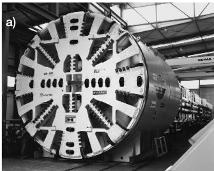
Figure 5.27 8.160 m diameter, 100 m long Herrenknecht S-192 Mixshield TBM used on the Channel Tunnel Rail Link (CTRL) project in the UK, a) before and b) at breakthrough. This machine drove through alluvium, chalk and flints (courtesy of Herrenknecht)
