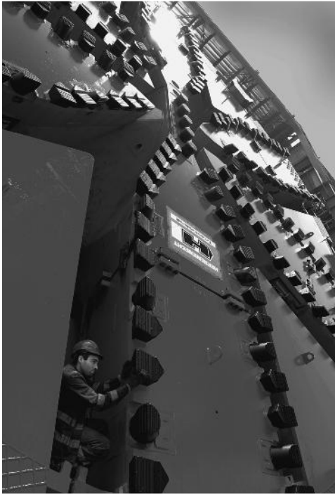
Figure 5.23 Cutter dressing used on a Mixshield TBM in Shanghai through sand, clay and loose gravel/boulders (courtesy of Herrenknecht)
