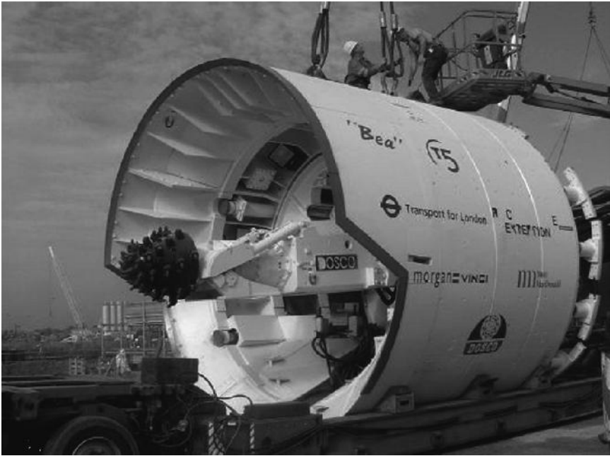
Figure 5.8 Refurbished Dosco boom-in-shield tunnelling machine as used for constructing the Piccadilly Line Extension (PiccEx) Tunnel to Heathrow Terminal 5 in the UK
