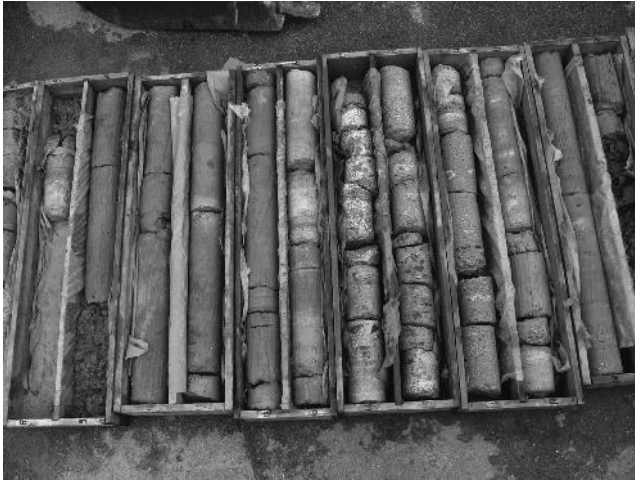
Figure 2.5 Example of continuous rock cores obtained from rotary drilling
