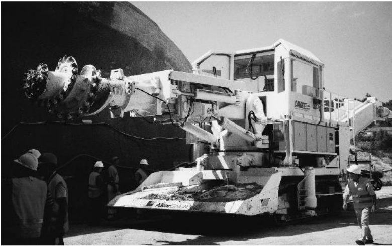
Figure 5.4 Partial face boring machine with an axial cutterhead (roadheader) (courtesy of Aker Wirth)
