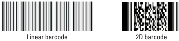
Figure 3.1 Linear and two-dimensional barcodes.
