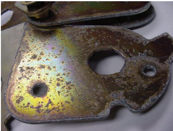
FIGURE 3.16 Pitting corrosion on galvanized steel.
