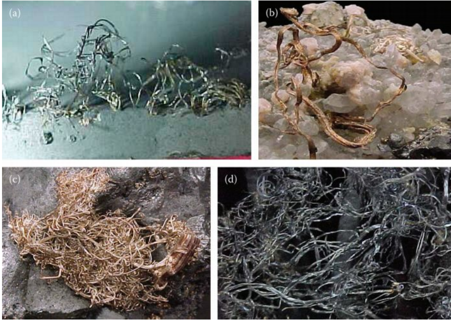
FIGURE 3.14 Corrosion silver whiskers and natural silver wires (a, b, c, and d): is there a difference?
