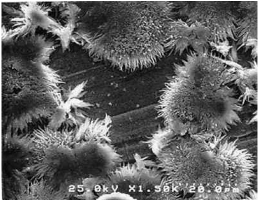
FIGURE 1.1 Sulfide-oxide “flowers” made of Cu, O, and S (×8000) cover the surfaces of silver-plated copper coupons after corrosion test.
