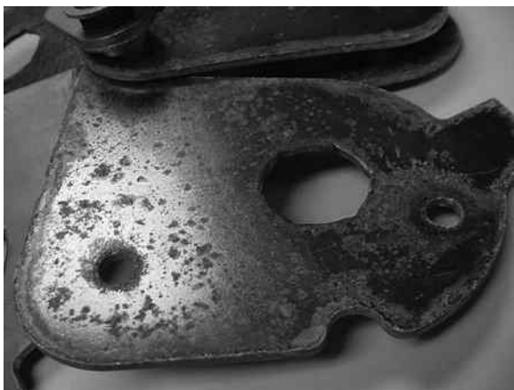
FIGURE 3.16 (See color insert.) Pitting corrosion on galvanized steel.
