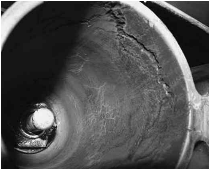
FIGURE 5.7 (See color insert.) PD damage on a cast resin CB spout. (From Neil D. Why PD measurement can pay dividends , Online. Available: http://www.pennenergy.com/index/power/display/8315670195/articles/power-engineering-international/volume-18/Issue_3/features/Why_partial_discharge_measurement_can_pay_dividends.html . With permission.)
