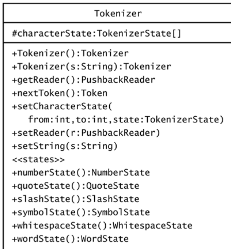
Figure 9.4. The Tokenizer class. A Tokenizer returns a series of tokens using various TokenizerState objects to build different types of tokens.
