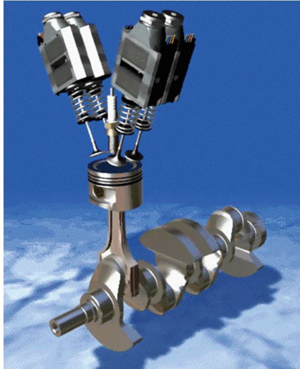
Fig. 2.34 Electromagnetic valves at intake and exhaust
