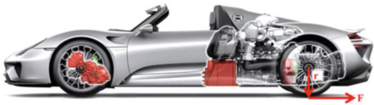
Fig. 1.22 Torque on the wheel of an automobile (Source: Stan, Porsche)
