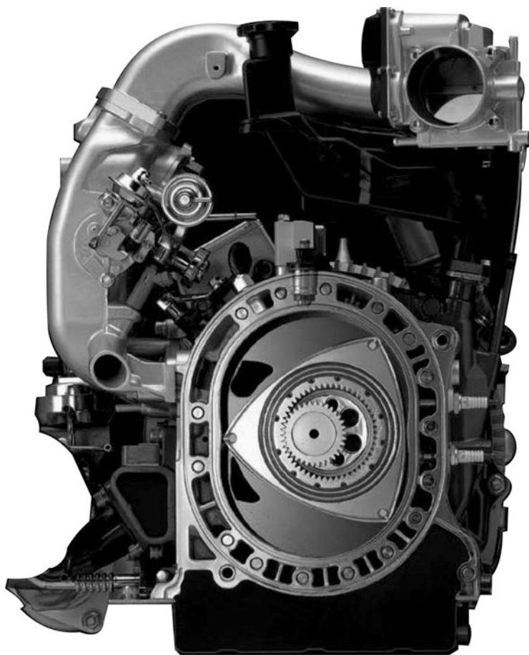
Fig. 2.87 Wankel engine with frontal intake and exhaust ports (Source: Mazda)
