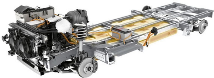
Fig. 4.13 Motor and battery topology in a heavy duty vehicle (Source: Daimler)
