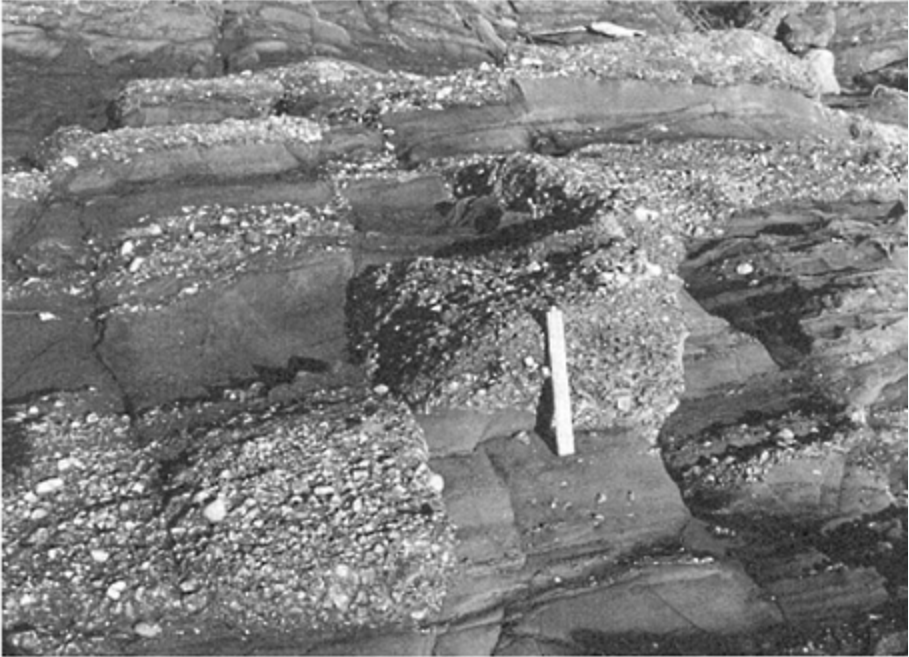
Figure 4.17 Layers of sandstone and conglomerate cut by small faults and joints (some of which are small shears) similar, apart from magnitude of displacement, to the faults. (Reproduced by kind permission of Dr Brian Bluck.)
