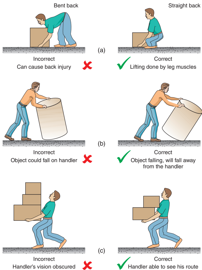
FIGURE 12.6 Lifting techniques.
