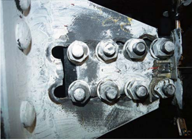
Figure 3.13 Laboratory test dramatically shows the block shear phenomenon. Source: Photo courtesy of J. Swanson and R. Leon, Georgia Tech.
