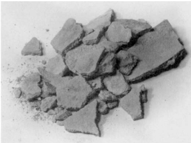
FIGURE 8.5.24 Mineral scale deposits of water minerals. (Courtesy of The Metro Group, Inc.)
