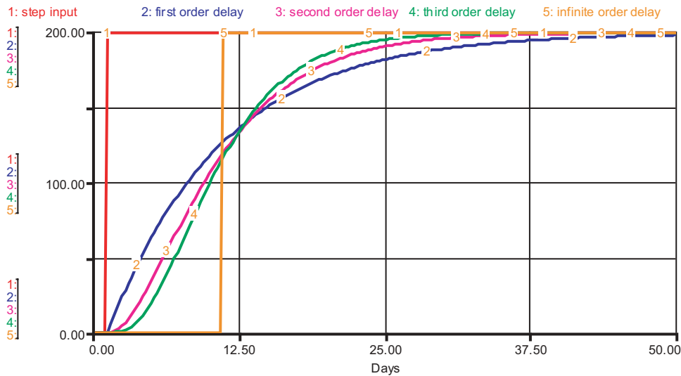
Figure 3.22. Delay responses to step input.
