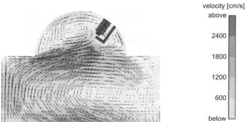
Fig. 6.15. Velocity field in a two-stroke DISI engine after scavenging
