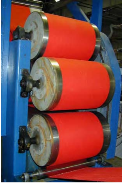
2.12 Steam heated drying cylinders.
