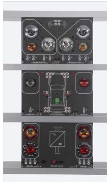
Experiment: "Vehicle lighting control via CAN bus" with a SO3216-2Z interface and additional components
