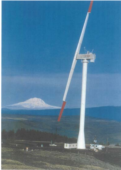
Fig. 3.10 American NASA MOD-2 machine 2.5 MW, 2-blade propeller.
