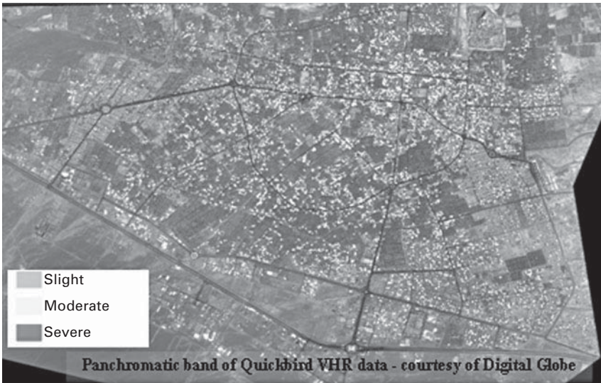
4.8 The damage detection results shown for the entire city.
