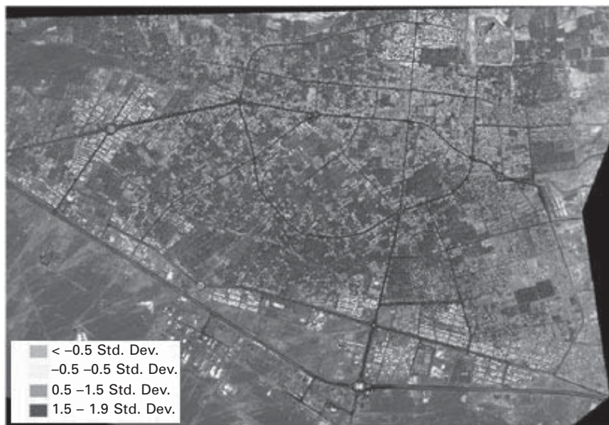
4.25 SAR change detection results (shown in Fig. 4.20) calibrated with the RCS orientation dependent curves.
