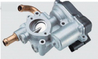
c) electrical exhaust valve, max. 700°C (2)
