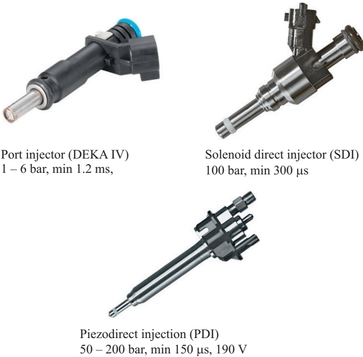
Fig. 5.4.3. Examples for gasoline injectors, Continental Automotive GmbH (2011).
