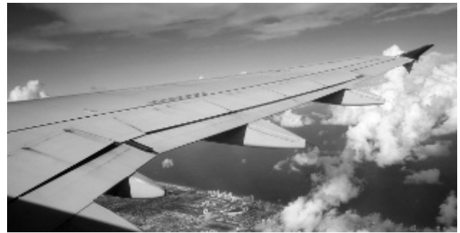
Figure 7.20: An airplane wing can be viewed as a tapered cantilever beam that is subject to aerodynamic and propulsive loading causing transverse vibration. (Photograph by M. Nagurka)
