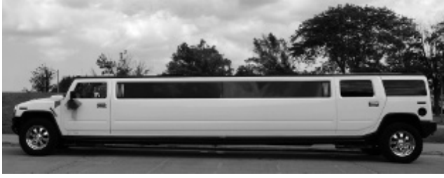
Figure 7.21: An extended Hummer would experience multiple modes of vibration. It can be modeled as a simply supported beam. (Milwaukee, WI; photograph by M. Nagurka)
