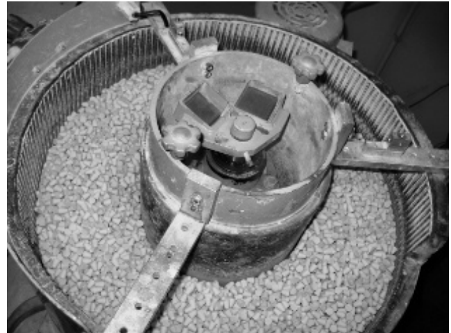
Figure 1.16: A vibratory bowl finisher (Spiratron ST-1, Roto-Finish, Kalamazoo, MI) in the Mass Finishing Laboratory, Marquette University. (Courtesy of Vikram Cariapa. Photograph by M. Nagurka)
