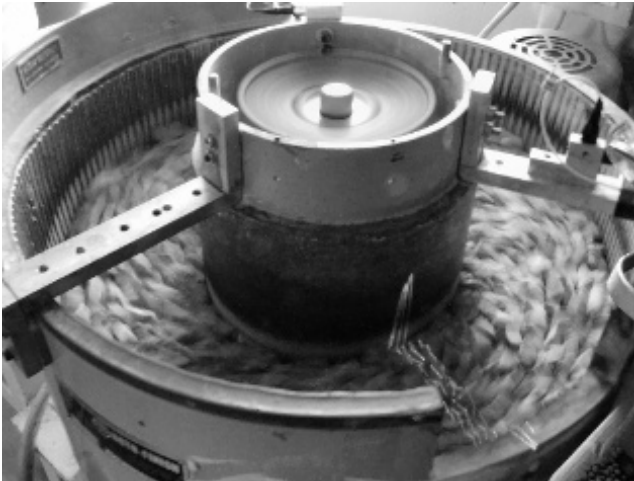
Figure 1.17: Vibratory bowl finishing in operation. Here a test was conducted to image the average dilated height of the media. It allowed the average density of the media to be determined during operation. (Courtesy of Thomas Silman and Vikram Cariapa. Photograph by T. Silman in the Mass Finishing Laboratory, Marquette University)
