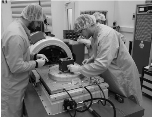
Figure 9.48: Installation of CubeSat OUFTI-1 on an electrodynamic shaker. The CubeSat, built by students at the Université de Liège, Belgium, complies to the CubeSat standard of 10 cm side length and a mass of 1 kg or less. The shaker is used to test the integrity of the CubeSat to simulate high vibration environments. (Courtesy European Space Agency)
