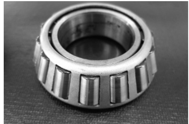
Figure 7.16: Rolling contact bearings, such as the tapered roller bearing shown, are used in rotating machinery. Many bearings fail prematurely because of contamination, poor lubrication, temperature extremes, poor fitting, unbalance, and misalignment. All of these factors lead to an increase in bearing vibration. To detect degrading bearings before they fail catastrophically (with the associated costs of downtime or damage to other parts of the machine), engineers often rely on “condition monitoring” software that indicates changes in acoustic emission or bearing temperature. (Photograph by M. Nagurka)
