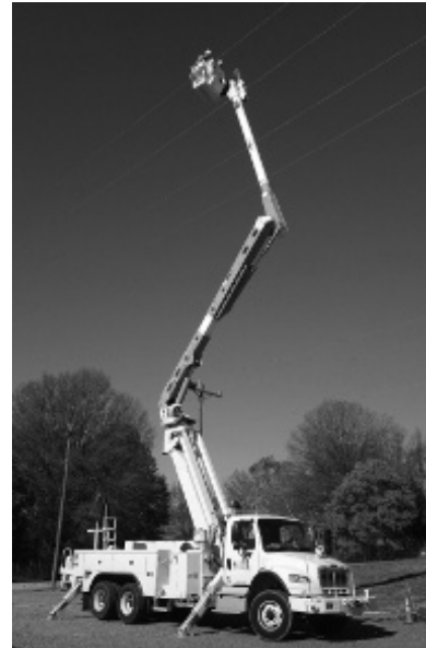
Figure 9.7: The aerial bucket on a boom truck can experience significant vibration due to motion for positioning as well as aerodynamic loading. (Charlotte, NC; photograph by M. Nagurka)
