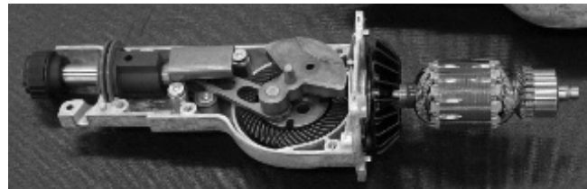
Figure 3.23: Internal mechanism of a Milwaukee Tool Sawzall that uses a slider-crank mechanism. The counterbalance on the crank is visible. (Courtesy of Mark Hickok, Milwaukee Electric Tool Corp.; photograph by M. Nagurka)
