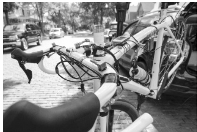
Figure 9.38: Accelerometers and data acquisition unit mounted to a bicycle. (Courtesy of Paul Harder, Trek Bicycle)
