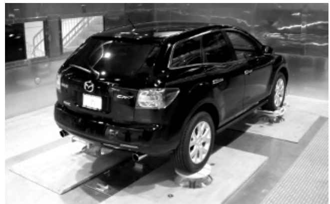
Figure 6.3: A Mazda CX-7 being tested on an MTS Model 320 7-Post Tire Coupled Road Simulator. (Courtesy Thomas R. Kurfess, May 2008)
