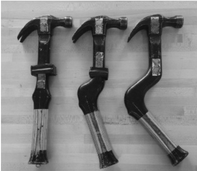
Figure 10.1: Redesigned hammers offer advantages in terms of attenuated vibration as well as ergonomics. Further advantages in terms of reduced vibration and weight can be achieved using titanium rather than steel. (Titanium has the same strength as steel with 45% less weight and exhibits much less vibration. Some hammer manufacturers claim up to 10 times less vibration.) (Ergonomics Laboratory, Marquette University; courtesy of Richard W. Marklin. Photograph by M. Nagurka)
