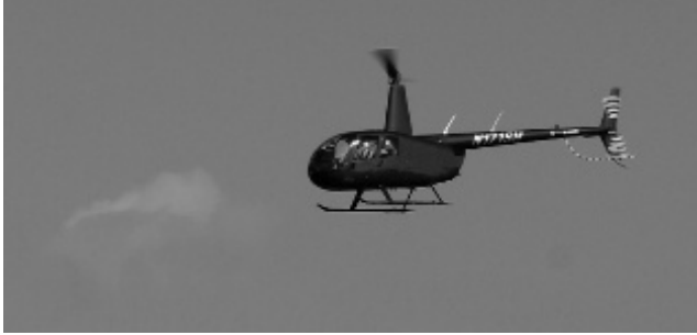
Figure 10.14: Vibration is a serious problem for rotorcraft designers. Not only debilitating to passengers and crew, vibration is detrimental to avionics and components, reducing reliability and life. The unsteady aerodynamics of rotor blades in forward flight produce vibratory loads that enter the hub, travel down to the gearbox and from there into the airframe. Traditionally, vibration has been reduced using absorbers placed in key locations—initially passive and tuned to a single rotor speed, but more recently active and able to adjust to variable speeds. (Milwaukee, WI; photograph by M. Nagurka)
