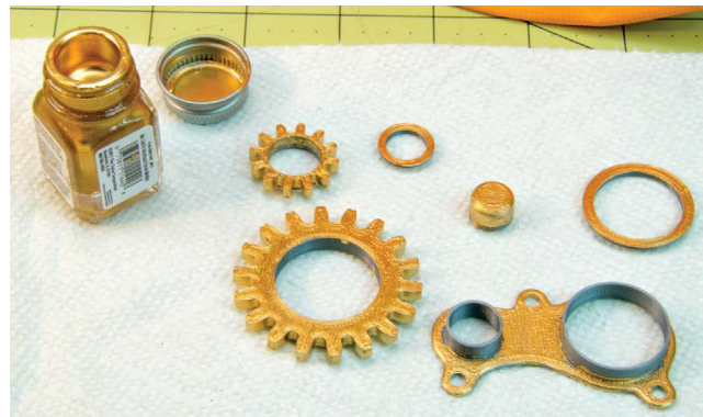
FIGURE 7-25: Dry the parts for two hours between coats
