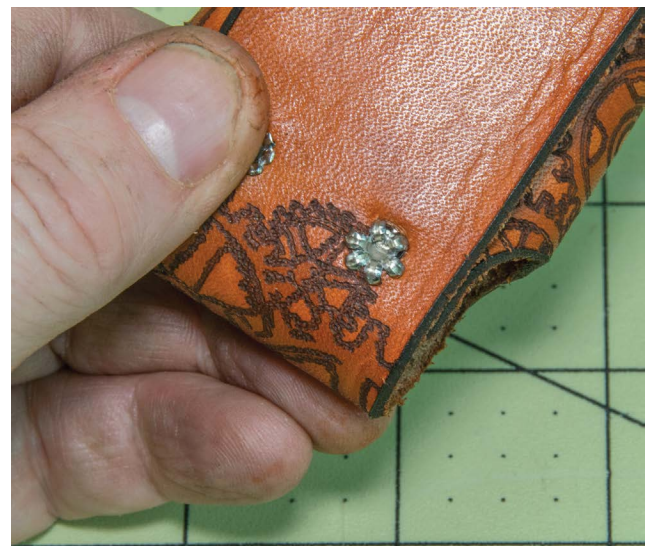
FIGURE 6-36: Correctly set tubular rivet
