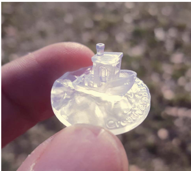
FIGURE 4-2: A 15 mm long 3DBenchy printed on a formlabs Form 2 IMAGE COURTESY OF WIKIMEDIA COMMONS
