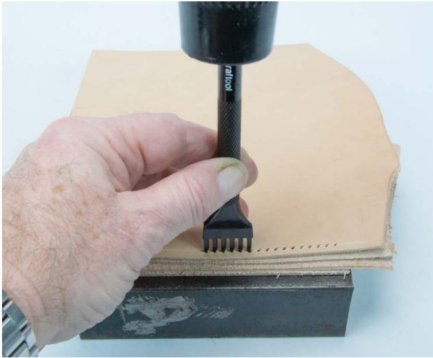
FIGURE 5-7: Manual stitching-hole creation
