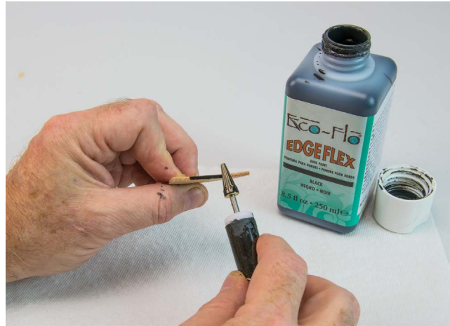
FIGURE 9-37: Edge coating with an edge roller
