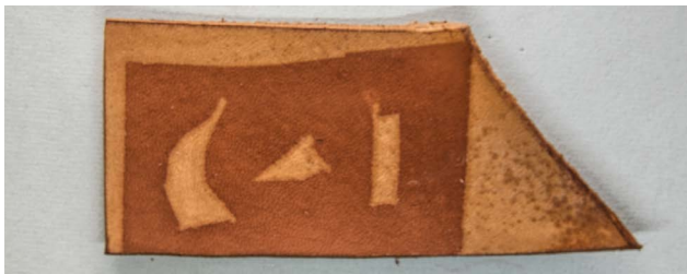
FIGURE 8-27: Resist that leaked around edges of vinyl stencil
