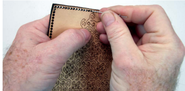
FIGURE 5-24: Clearing the stitching holes
