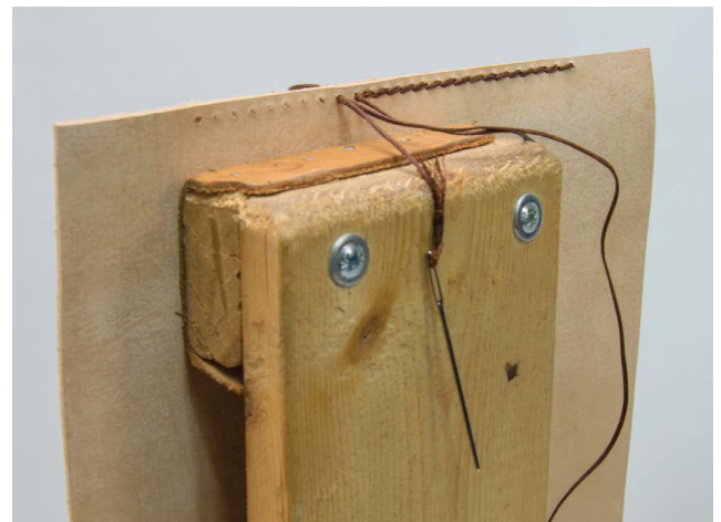
FIGURE 9-24: Stitched reinforcement holes
