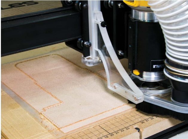
FIGURE 10-21: Holes and outline completed
