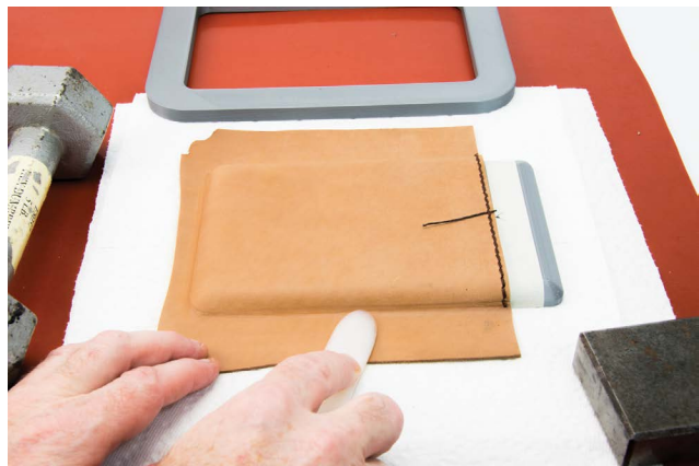
FIGURE 9-26: Smoothing out the molding
