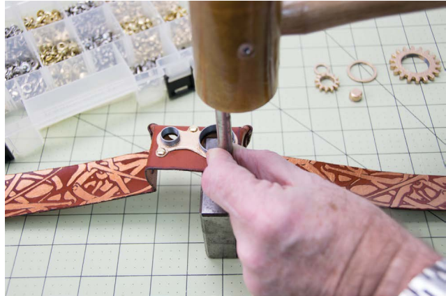
FIGURE 7-28: Setting the Rapid Rivets
