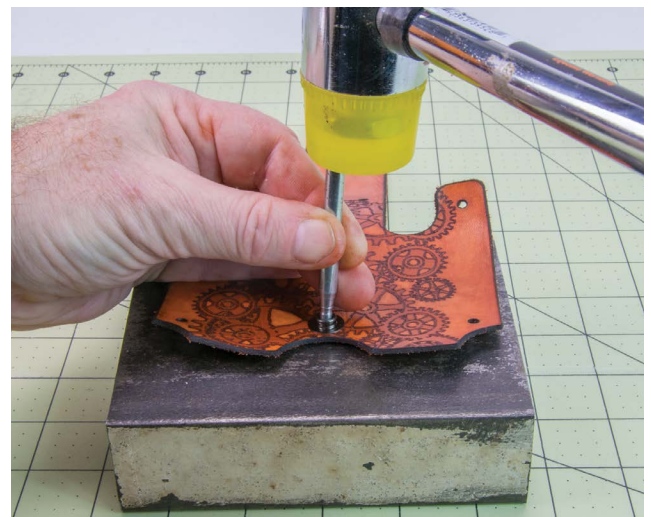
FIGURE 6-32: Setting the stud
