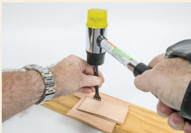
FIGURE 2-42: Punching the holes
