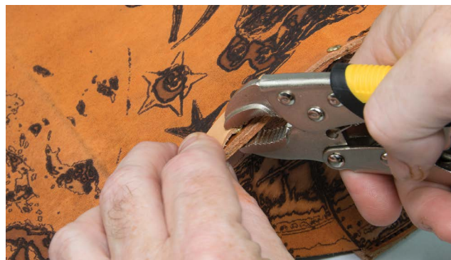
FIGURE 11-36: Riveting the holes on the upper section
