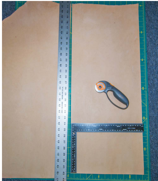
FIGURE 11-15: Manually cutting out the rough main body
