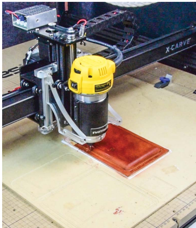
FIGURE 9-31: Milling and drilling the top and bottom pieces
