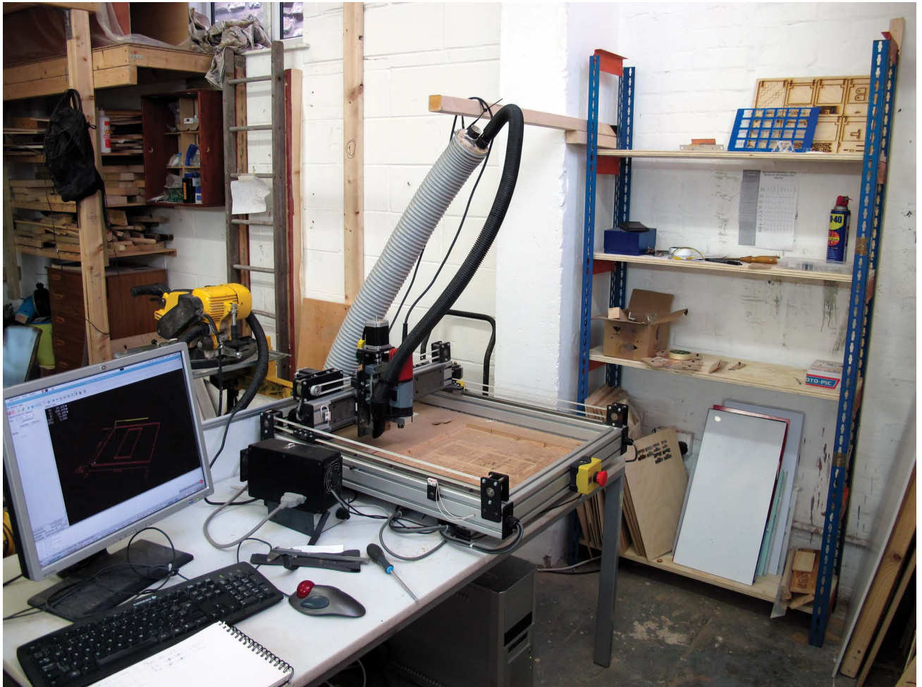
FIGURE 3-2: CNC router in a workshop IMAGE COURTESY OF WIKIMEDIA COMMONS
