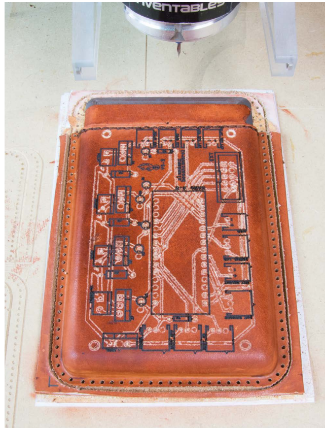
FIGURE 9-35: Burning the silkscreen layer
