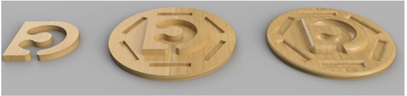
FIGURE 3-3: Machining in 2D, 2.5D, and 3D
