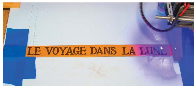
FIGURE 11-20: Burning the strap
