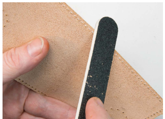
FIGURE 8-33: Filing off unwanted fibers
