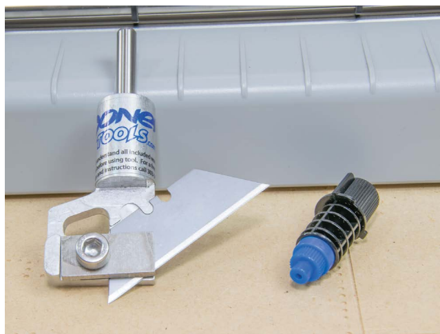
FIGURE 8-23: CNC drag knife vs. stencil cutter knife
