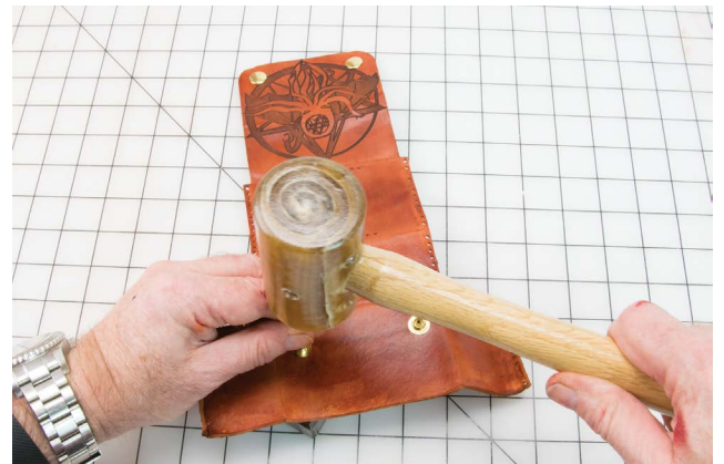
FIGURE 10-29: Setting the snaps
