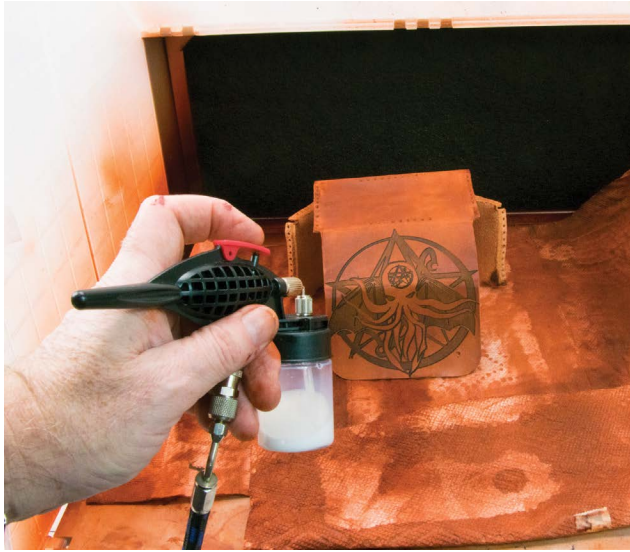
FIGURE 10-27: Dyeing the pouch
