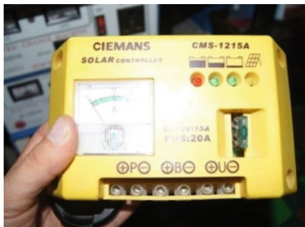
Fig. 14.2 A “Ciemens” charge controller (courtesy of P. Dauenhauer)
