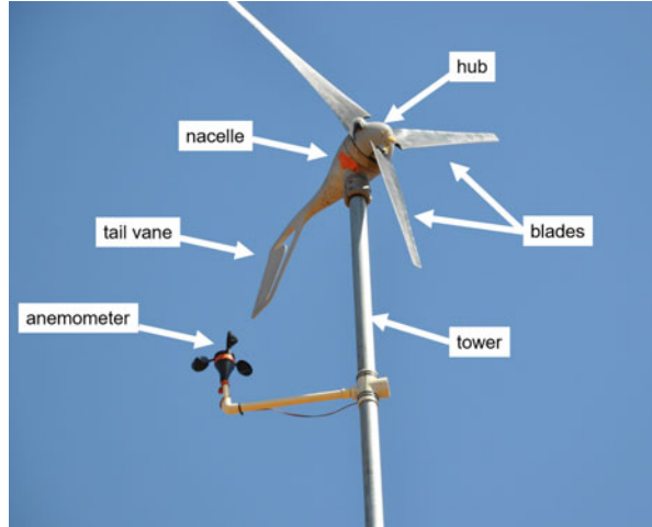
Fig. 6.1 A 400 W three-blade horizontal axis wind turbine with blade length of 0.5 m. An anemometer is used to measure the wind speed
