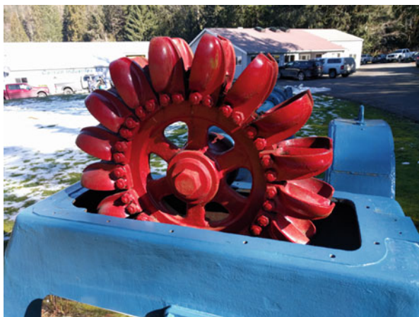
Fig. 6.21 A large horizontal axis Pelton turbine with its casing and manifold removed. This turbine has been decommissioned and its buckets painted. It serves as a display model. It is larger than would typically be found in MHP systems (courtesy of the author)
