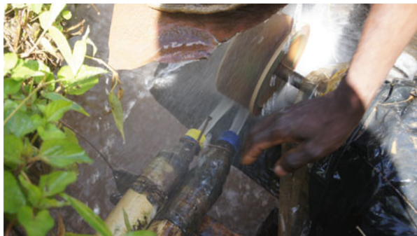
Fig. 6.27 An improvised hydroturbine in Malawi. Notice the use of plastic beverage bottles for nozzles (courtesy P. Dauenhauer)
