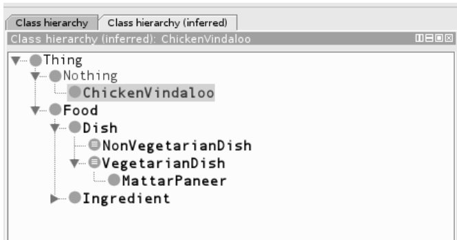
FIGURE 4.7: Protégé Tutorial (4). ChickenVindaloo has been inferred to be a subclass of Nothing because it is unsatisfiable.
