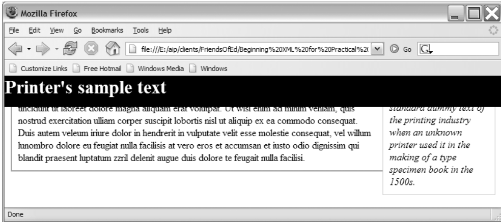
Figure 5-14. Fixed content appears on top of the other elements in the XML document.
