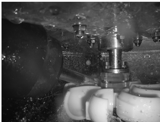
Figure 2.6: Turgo Turbine Case Study – FDM Rapid Prototyped Component under Experimental Testing.
