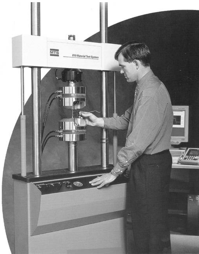
FIGURE 3.13 Servohydraulic testing machine. (Courtesy of the MTS Systems Corporation, Eden Prairie, MN.)
