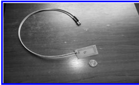
FIGURE 6.46 Loop antenna for RFID applications.
