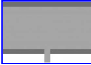
FIGURE 3.8 A microstrip stacked patch antenna.
