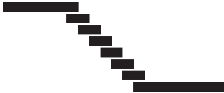
FIGURE 10.28 Edge coupled filter.
