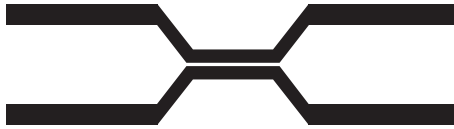
FIGURE 10.29 Single-layer microstrip directional coupler.
