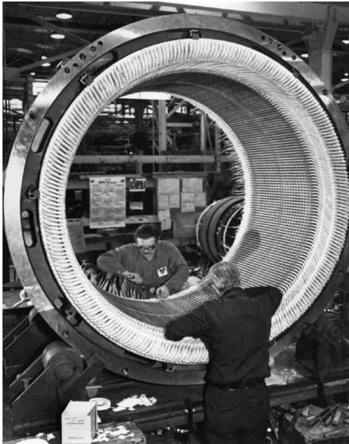
FIGURE 7.4 Winding the stator of a synchronous generator. (Courtesy of MagneTex, Nashville, TN.)
