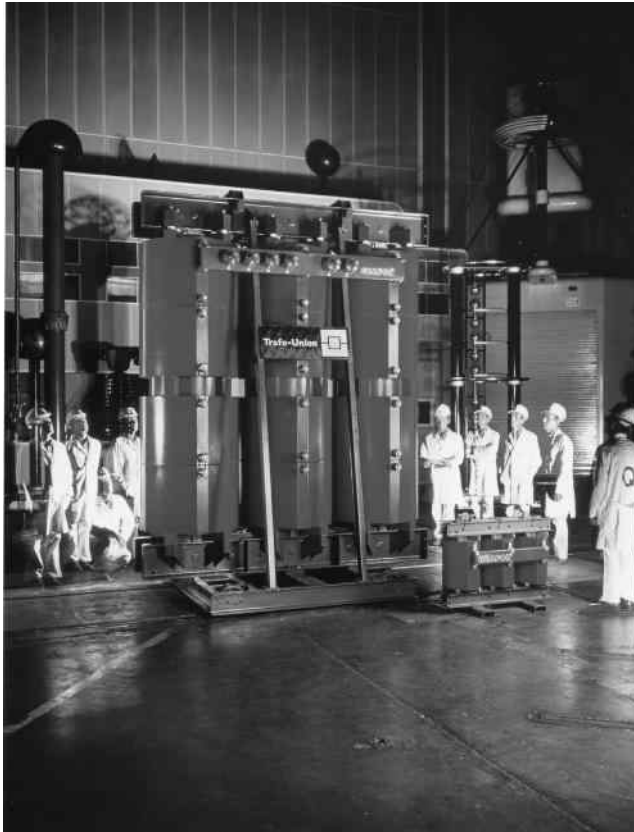
FIGURE 4.27 (See color insert.) 10 MVA and 50 kVA, core-type, three-phase transformers with GEA FOL solid dielectric cores. (Courtesy of Siemens AG, Munich, Germany.)
