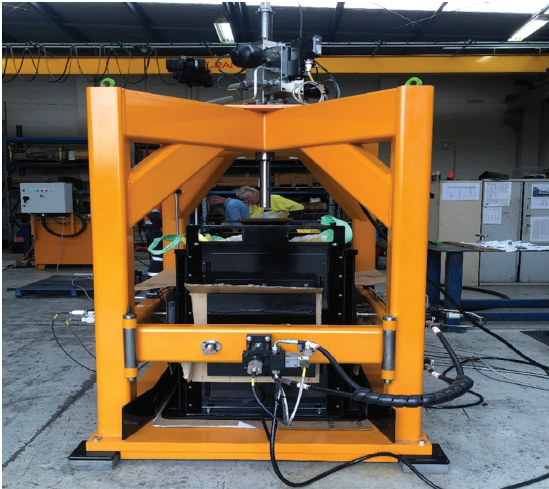
Figure D2 Large-scale process simulation triaxial facility. Sample size: 600 \times 800 mm in area and 1 m in depth.
