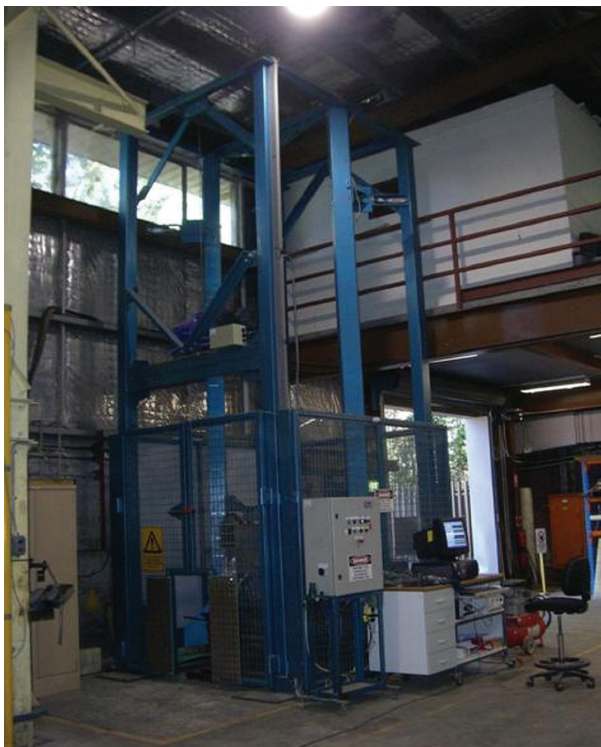
Figure D5 Impact testing machine. Drop height: 8 m, sample size: 300 mm in diameter and 600 mm high.
