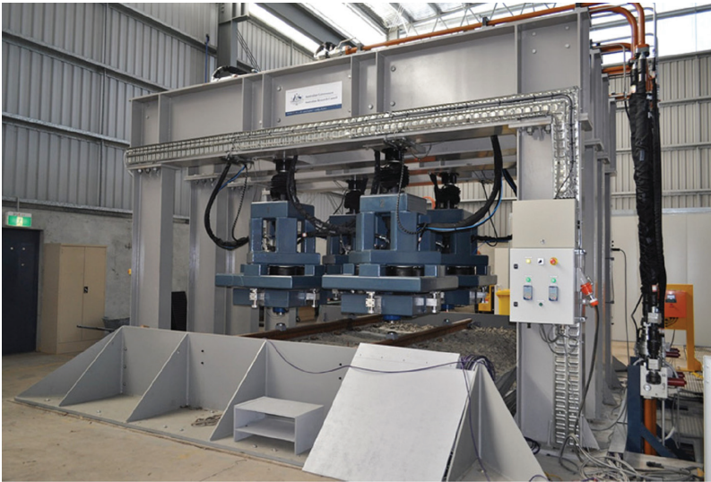
Figure D4 National facility for cyclic testing of high-speed rail (FCTHSR), cross section: 4 \times 4 \text{ m}^2 , depth: 2 m.
