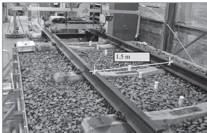
Figure 13.3 The completed model track with sleepers and rails on it (Su et al. [1]).
