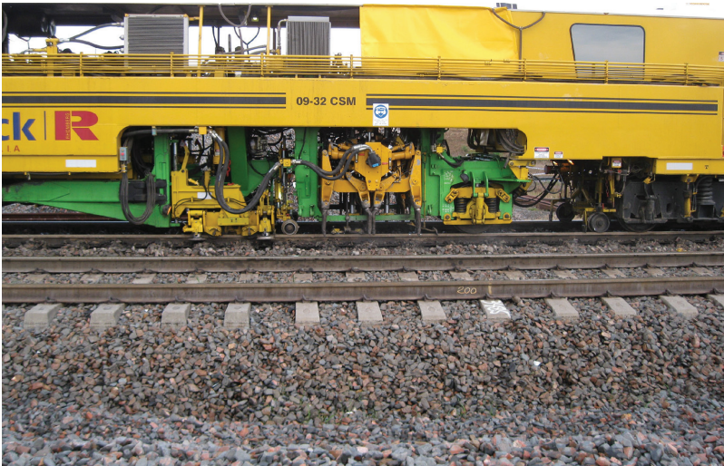
Figure C3 Automated tamping equipment used at fully instrumented track at Singleton town near Newcastle, New South Wales.
