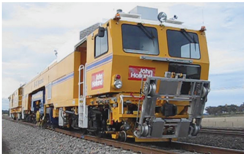
Figure 14.1 A typical tamping machine used for track maintenance.
