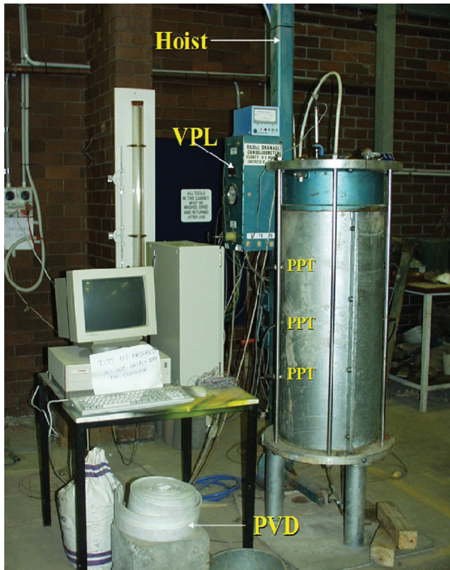
Figure D8 Large-scale consolidometer. Sample size: 700 mm in diameter and 1,000 mm high.
