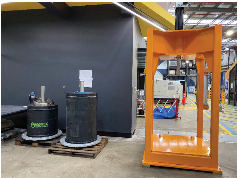
Figure D3 Large-scale cyclic triaxial apparatus. Sample size: 500 mm in diameter and 1,000 mm high.
