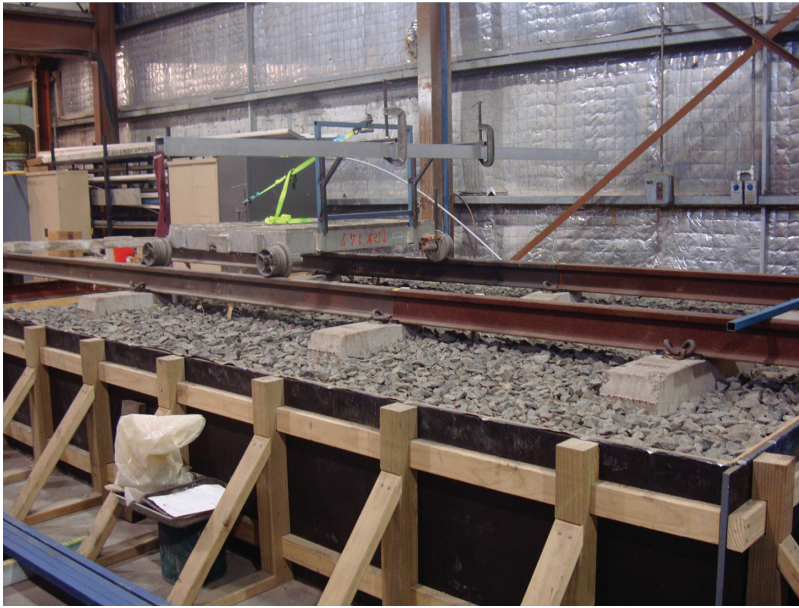
Figure D6 Model track used for non-destructive testing. Cross section: 4 \times 6 \text{ m}^2 , depth: 1 m.
