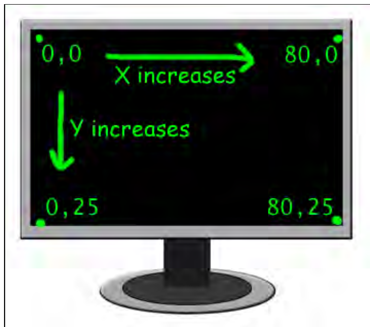
Figure 12-12: The Cartesian coordinate system on a computer monitor.
