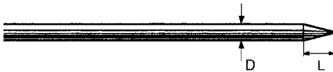
Figure 3.7 Normally the tip of the electrode is ground to a length L = 1.5-2 times the diameter ( D ).
