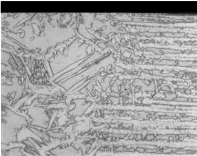
Figure 14.16 Microstructure of the weld metal and the HAZ in ferritic-austenitic steel.
