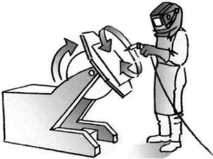
Figure 5.22 A positioner for the workpiece.
