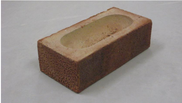
Fig. 30 Frogged brick (facing).
