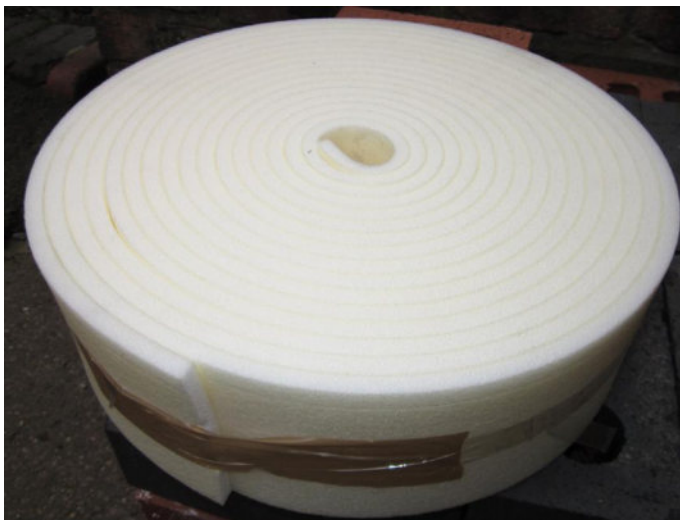
Fig. 48 Roll of polyethylene expansion joint foam.
