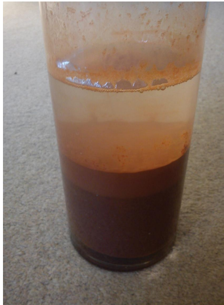
Fig. 22 Result of a field settling test carried out on soft sand.
