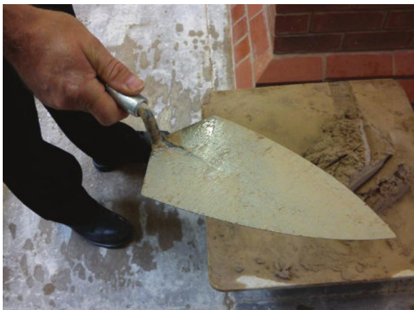
Fig. 106 Correct method of holding the trowel.
