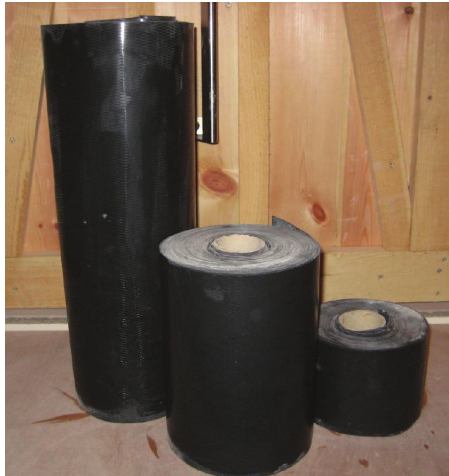
Fig. 168 DPC felt in different roll widths.
