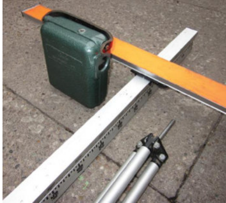
Fig. 58 Cowley Automatic Level, tripod, staff and target.
