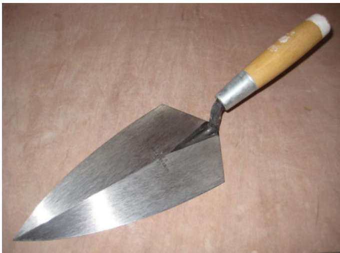
Fig. 61 Philadelphia Pattern brick trowel.
