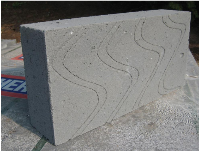
Fig. 37 Aerated concrete block.
