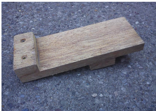
Fig. 147 Wooden closer gauge, also known as a bat gauge.
