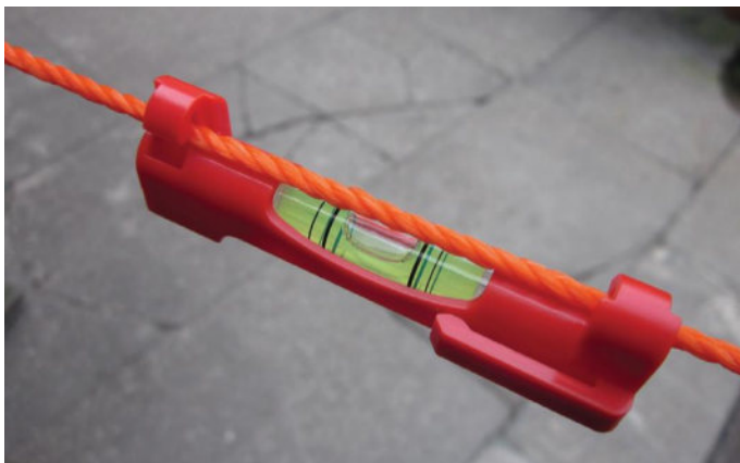
Fig. 52 Line-level attached to the ranging line.
