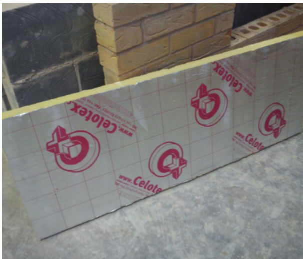
Fig. 175 Rigid foam insulation, or partial-fill cavity insulation.
