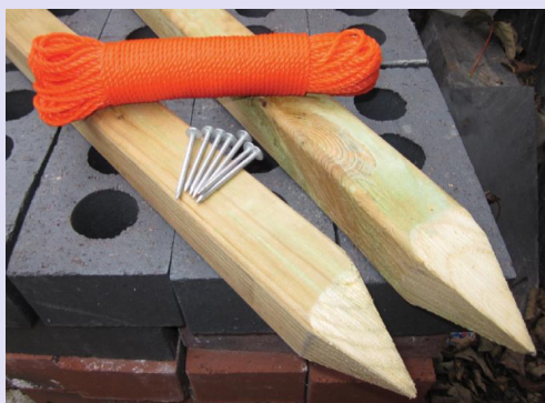
Fig. 49 Wooden pegs, ranging line and clout nails.
