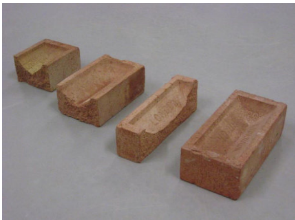
Fig. 145 Half bat, three-quarter bat, Queen Closer and full brick.
