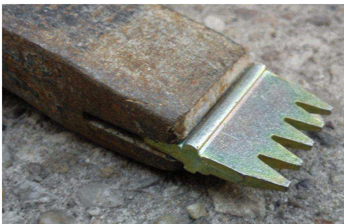
Fig. 75 Head of a scutch hammer showing the replaceable comb.
