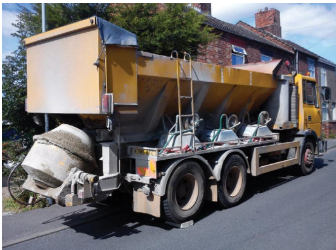
Fig. 14 Lorry delivering 'mini-mix' concrete.
